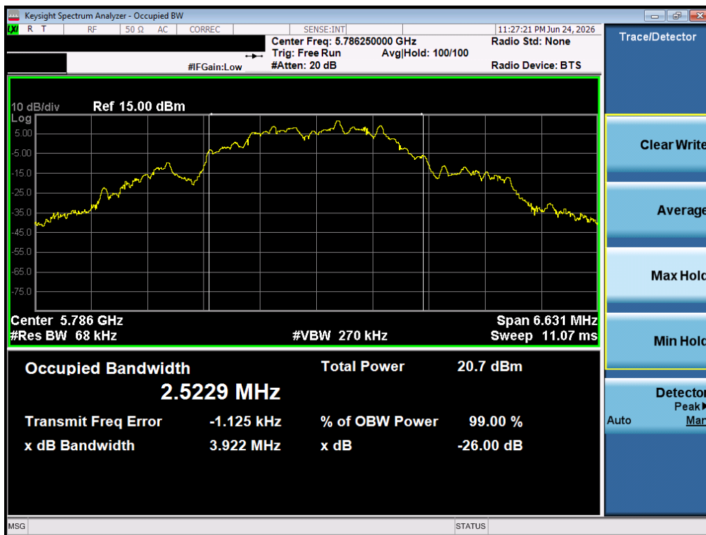
Plot 7-8. 99% OBW (O-QPSK, 5786.25MHz, 1000kbps)
