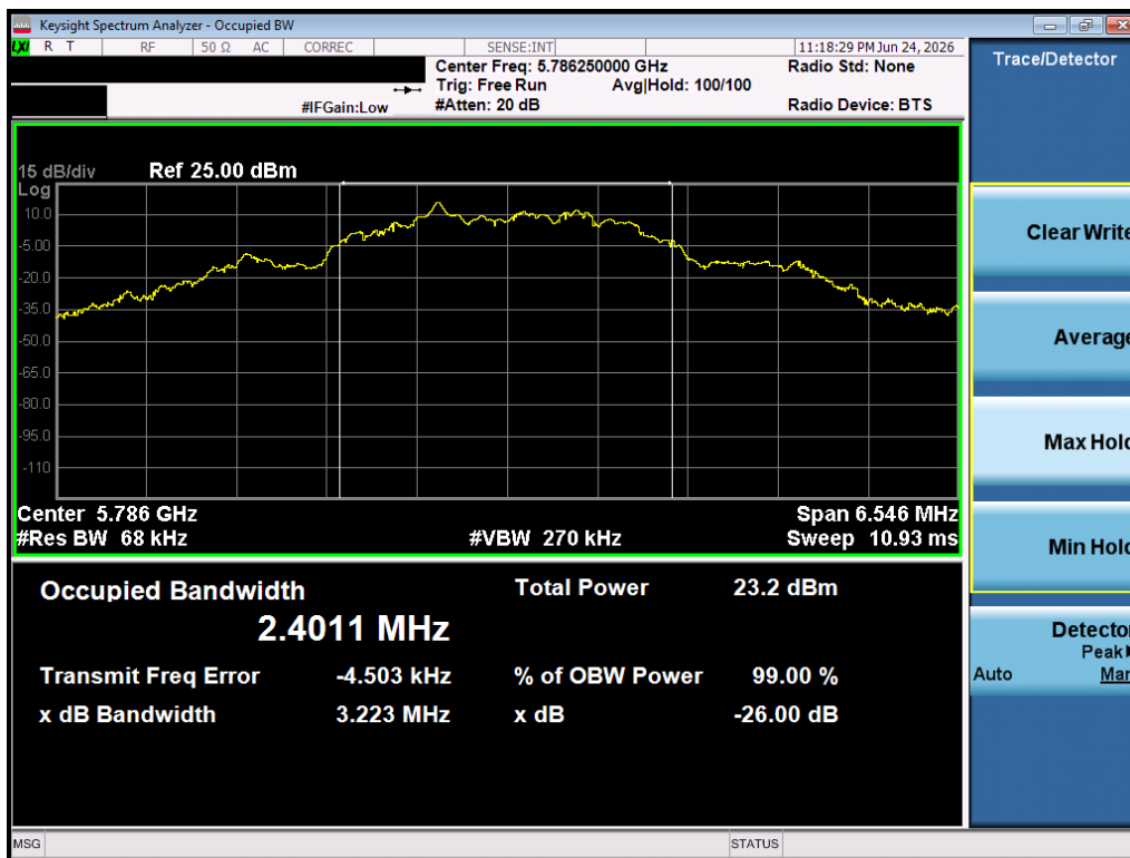
Plot 7-5. 99% OBW (O-QPSK, 5786.25MHz, 500kbps)
