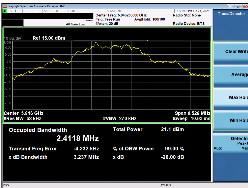
Plot 7-6. 99% OBW (O-QPSK, 5846.25MHz, 500kbps)
