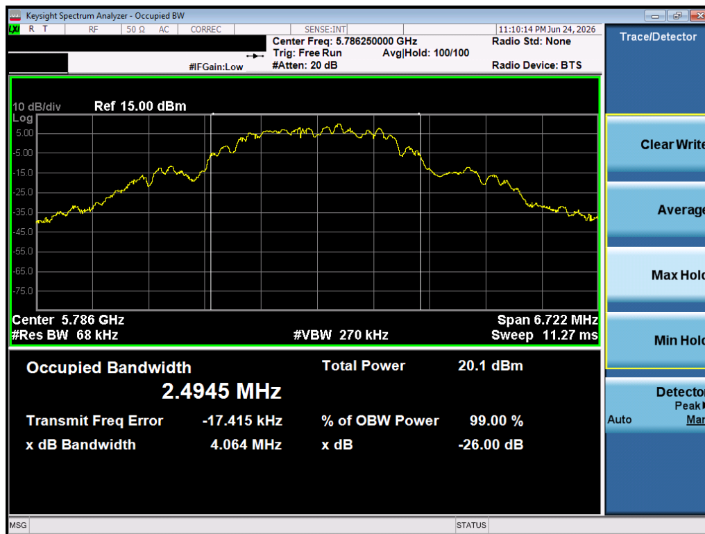
Plot 7-2. 99% OBW (O-QPSK, 5786.25MHz, 250kbps)
