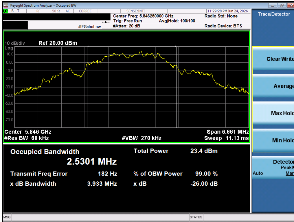
Plot 7-9. 99% OBW (O-QPSK, 5846.25MHz, 1000kbps)
