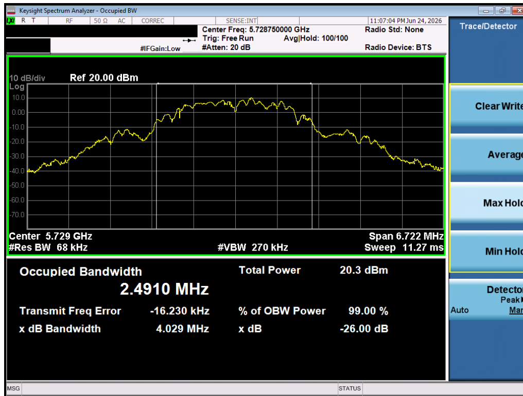
Plot 7-1. 99% OBW (O-QPSK, 5728.75MHz, 250kbps)
