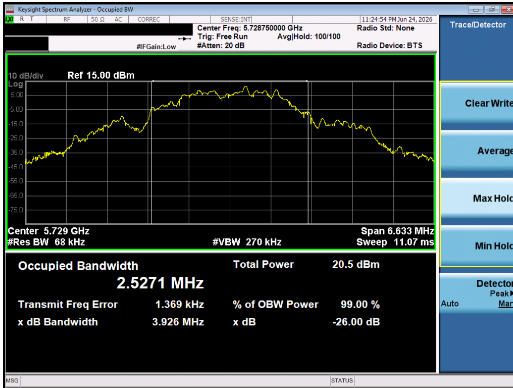
Plot 7-7. 99% OBW (O-QPSK, 5728.75MHz, 1000kbps)
