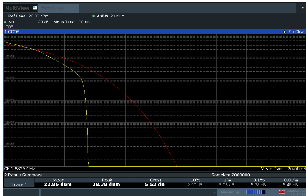
Plot 7-134. PAR Plot (LTE Band 25 - 20MHz 16-QAM - Full RB Configuration)
