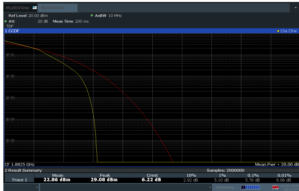
Plot 7-130. PAR Plot (LTE Band 25 - 10MHz 16-QAM - Full RB Configuration)
