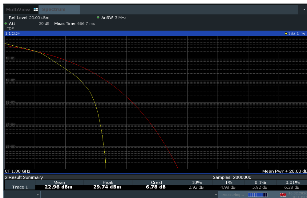
Plot 7-138. PAR Plot (LTE Band 2 - 3MHz 16-QAM - Full RB Configuration)
