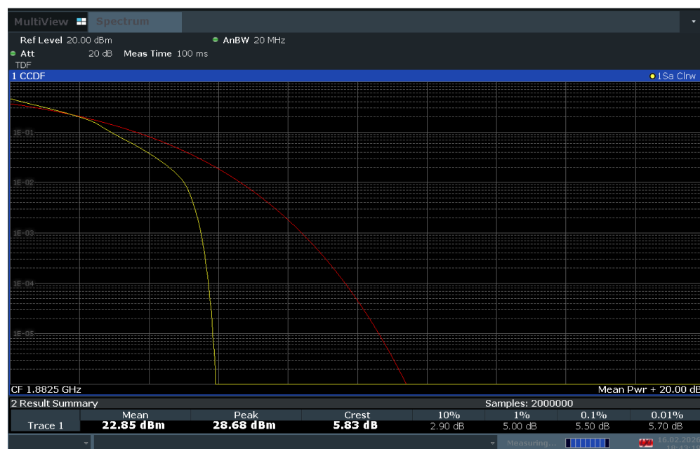
Plot 7-132. PAR Plot (LTE Band 25 - 15MHz 16-QAM - Full RB Configuration)
