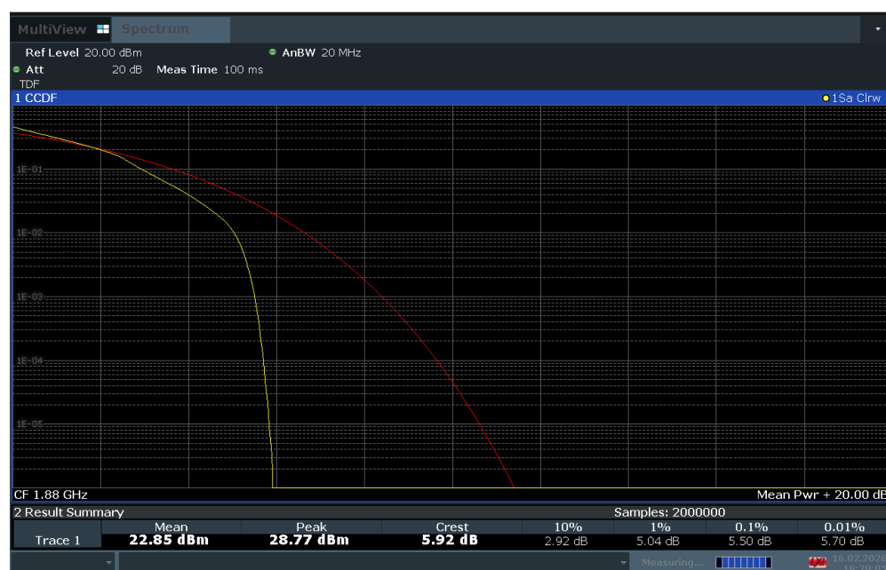
Plot 7-144. PAR Plot (LTE Band 2 - 15MHz 16-QAM - Full RB Configuration)
