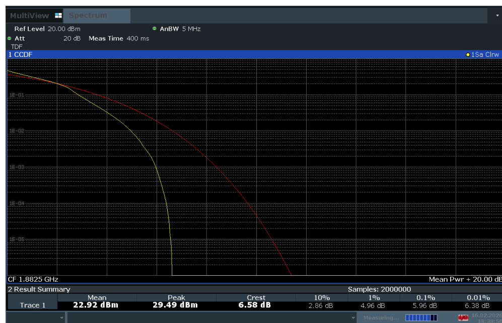
Plot 7-128. PAR Plot (LTE Band 25 - 5MHz 16-QAM - Full RB Configuration)
