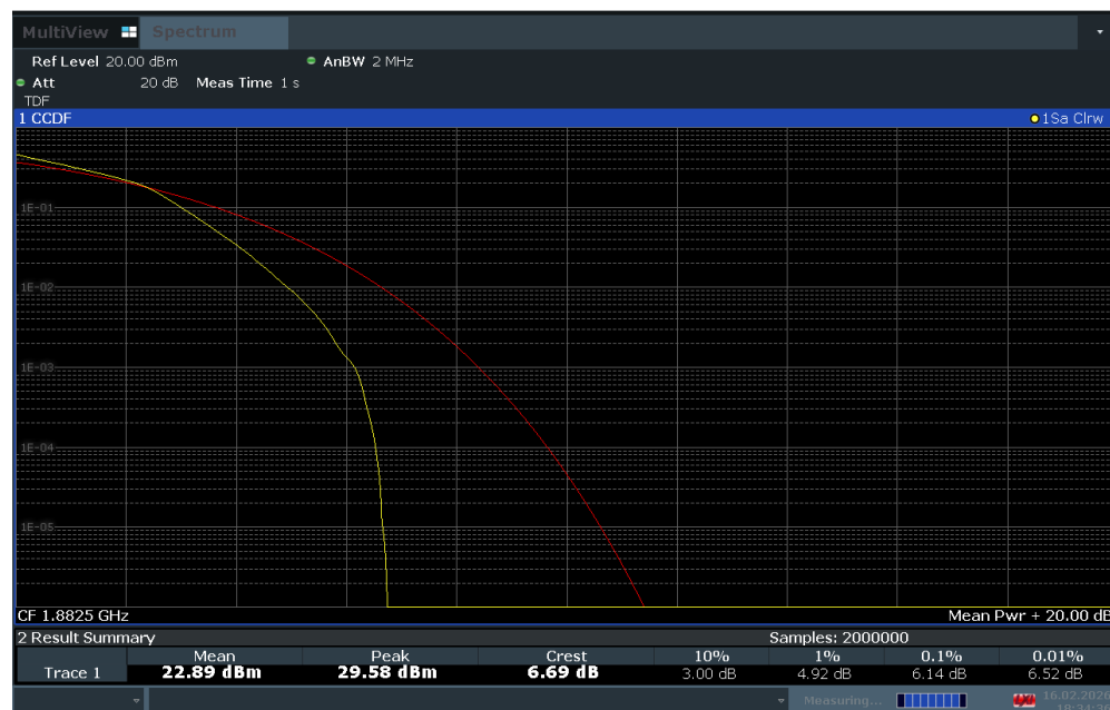
Plot 7-124. PAR Plot (LTE Band 25 - 1.4MHz 16-QAM - Full RB Configuration)
