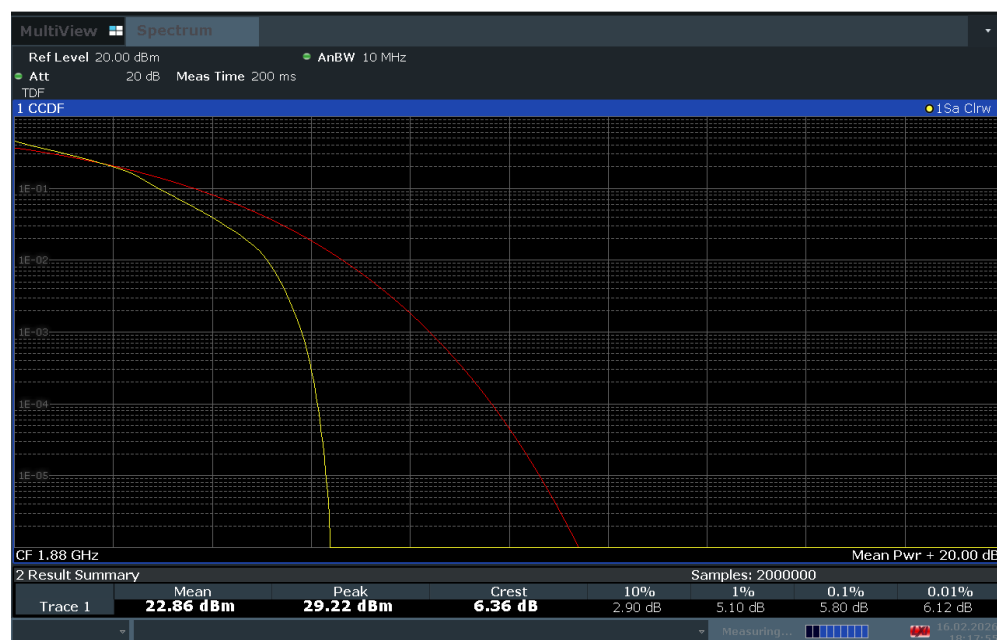
Plot 7-142. PAR Plot (LTE Band 2 - 10MHz 16-QAM - Full RB Configuration)
