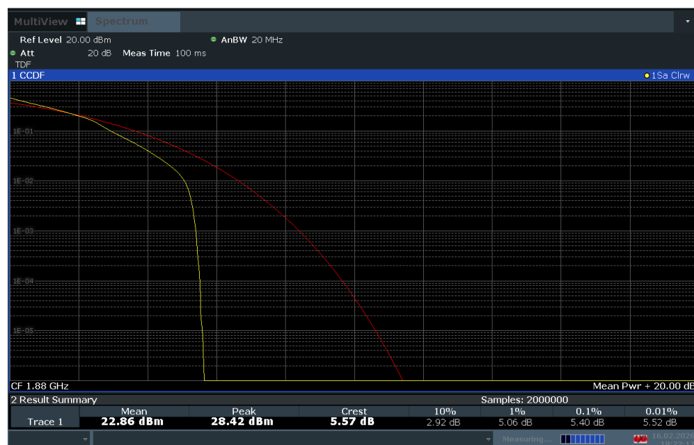
Plot 7-146. PAR Plot (LTE Band 2 - 20MHz 16-QAM - Full RB Configuration)
