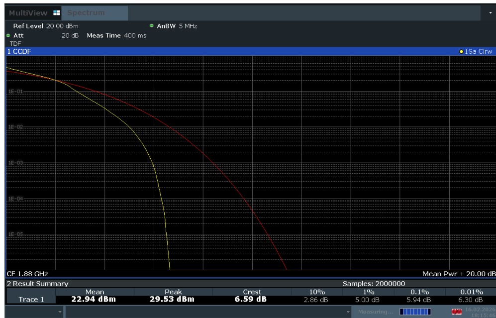
Plot 7-140. PAR Plot (LTE Band 2 - 5MHz 16-QAM - Full RB Configuration)
