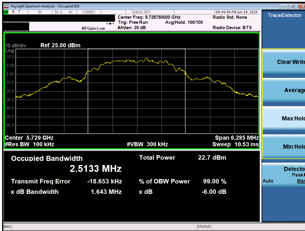
Plot 7-10. 6dB BW (O-QPSK, 5728.75 MHz, 250kbps)
