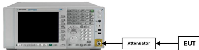
Figure 7-2. Test Instrument & Measurement Setup
