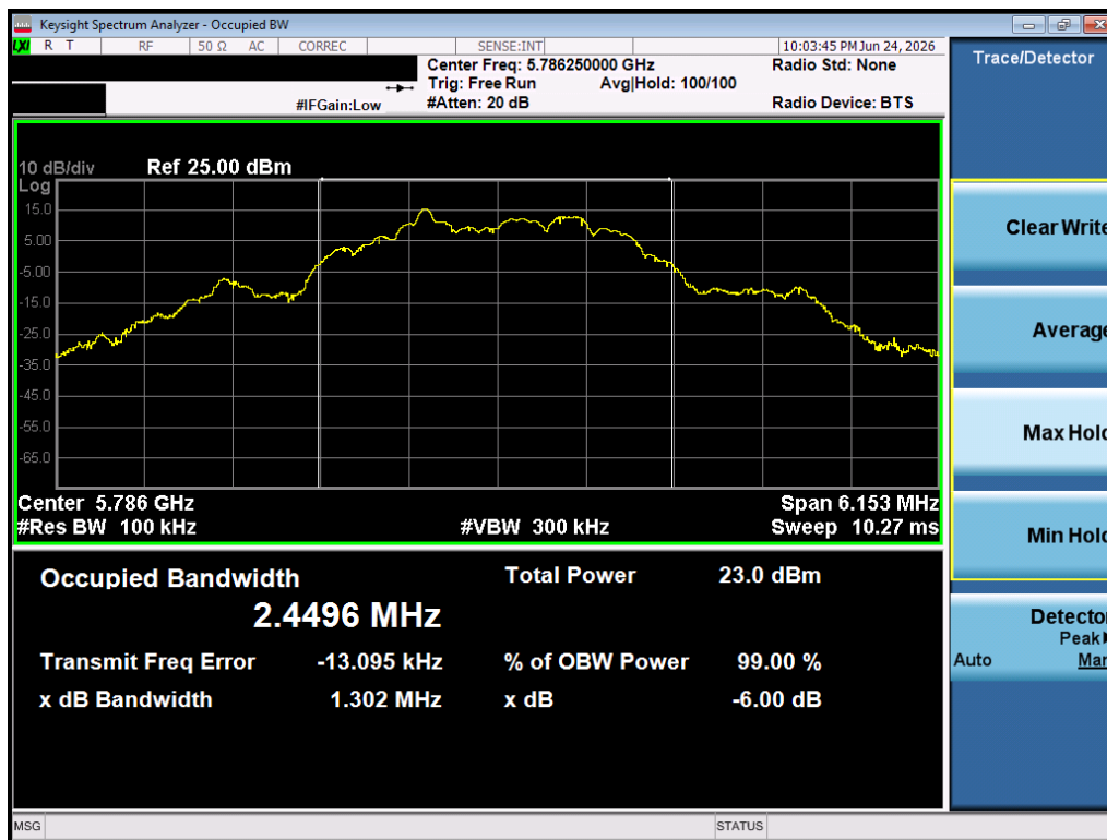
Plot 7-14. 6dB BW (O-QPSK, 5786.25 MHz, 500kbps)
