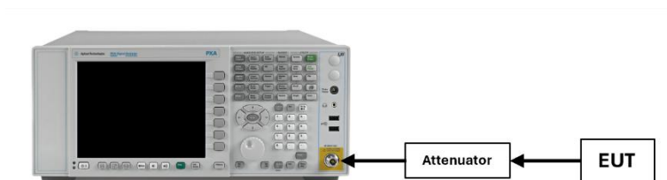
Figure 7-1. Test Instrument & Measurement Setup
