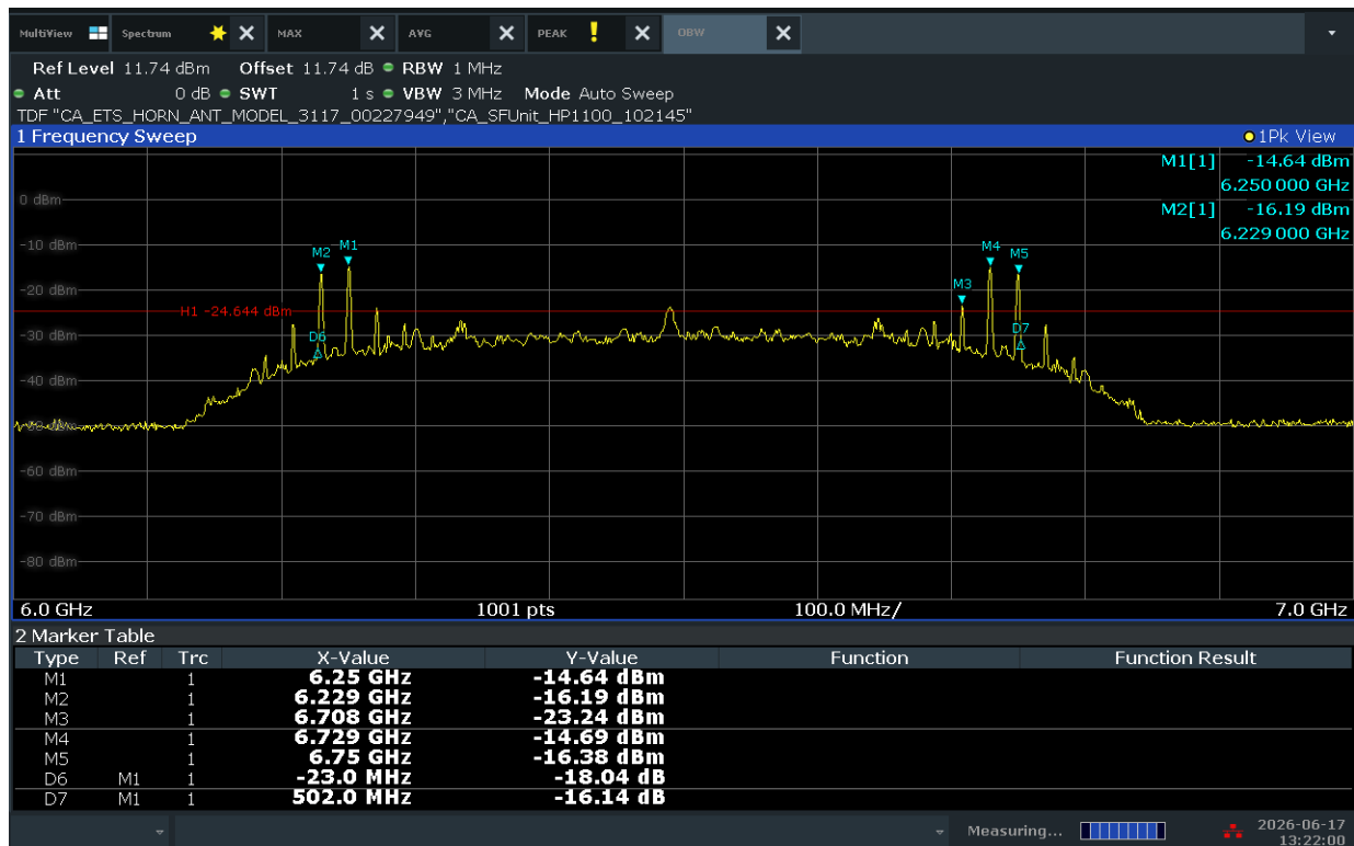
Plot 7-1. 10dBc Bandwidth (Ch. 5, Config 9/Payload 125B)
