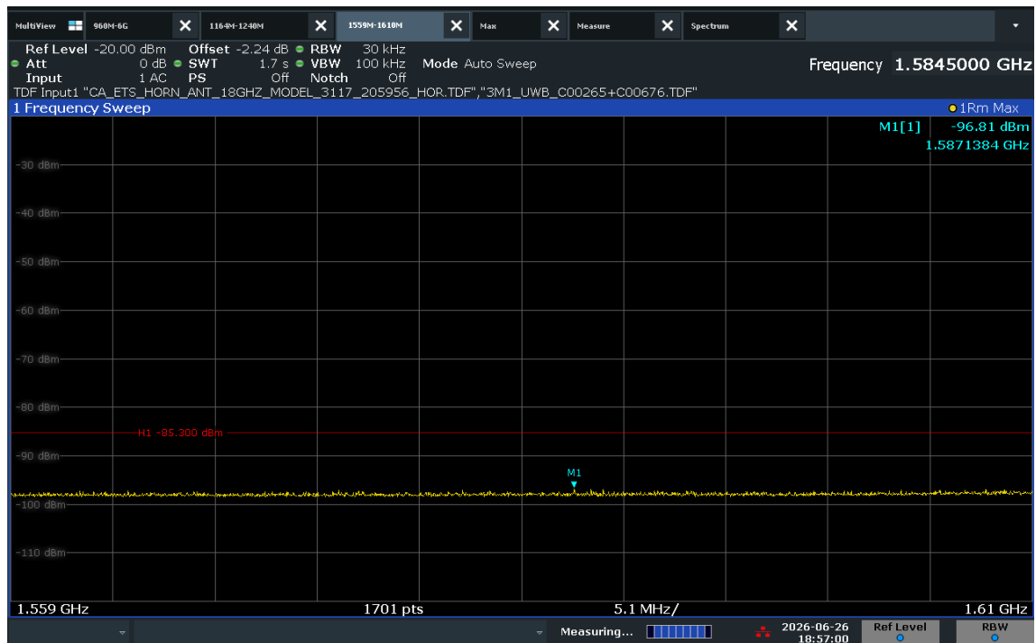
Plot 7-20. Radiated Spurious Emission 1559-1610MHz (Ch. 5, Config 9, Payload 125B Ant. Pol. H/V)
