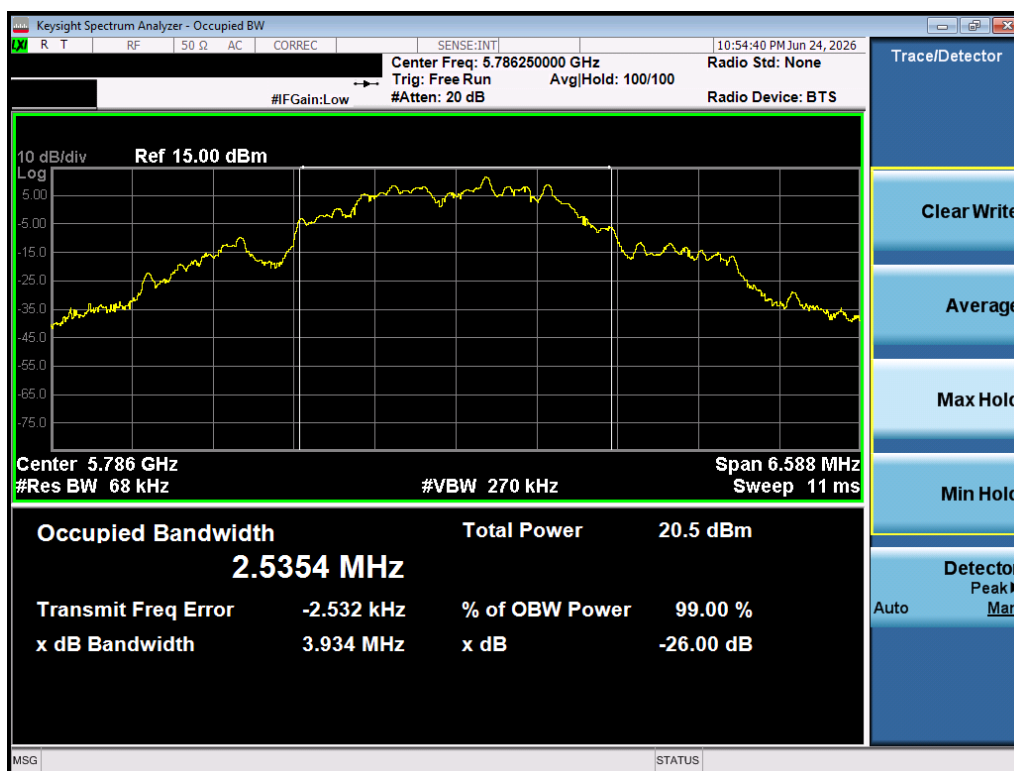
Plot 7-8. 99% OBW (O-QPSK, 5786.25 MHz, 1000kbps)
