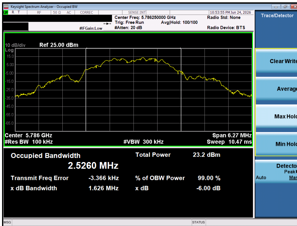
Plot 7-17. 6dB BW (O-QPSK, 5786.25 MHz, 1000kbps)
