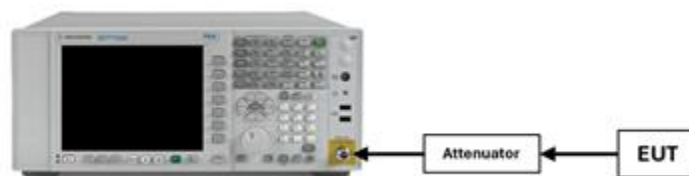
Figure 7-4. Test Instrument & Measurement Setup
