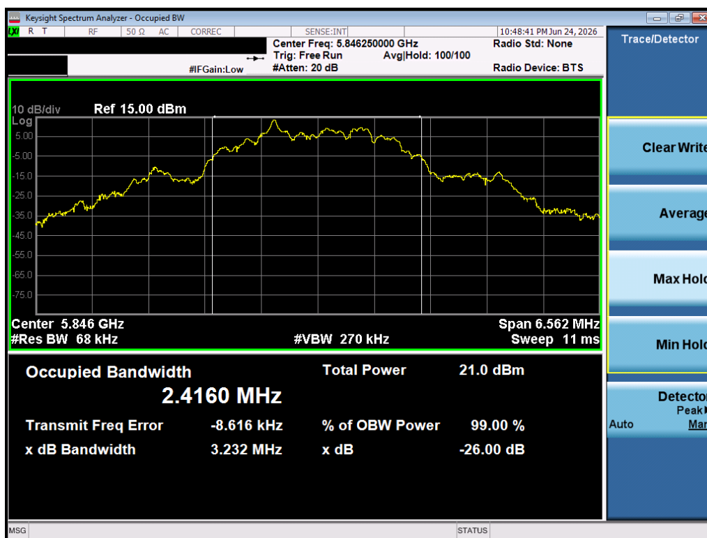
Plot 7-6. 99% OBW (O-QPSK, 5846.25 MHz, 500kbps)
