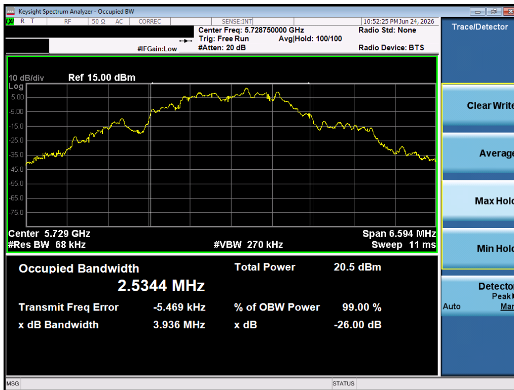
Plot 7-7. 99% OBW (O-QPSK, 5728.75 MHz, 1000kbps)
