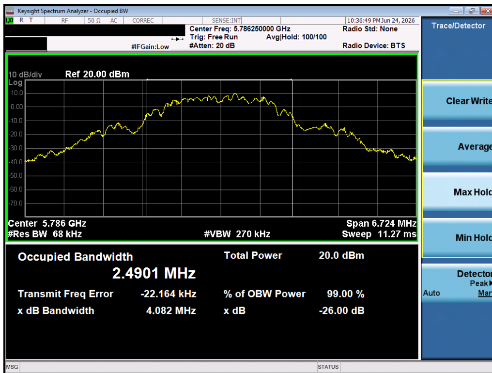
Plot 7-2. 99% OBW (O-QPSK, 5786.25 MHz, 250kbps)
