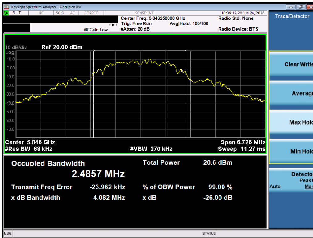
Plot 7-3. 99% OBW (O-QPSK, 5846.25 MHz, 250kbps)
