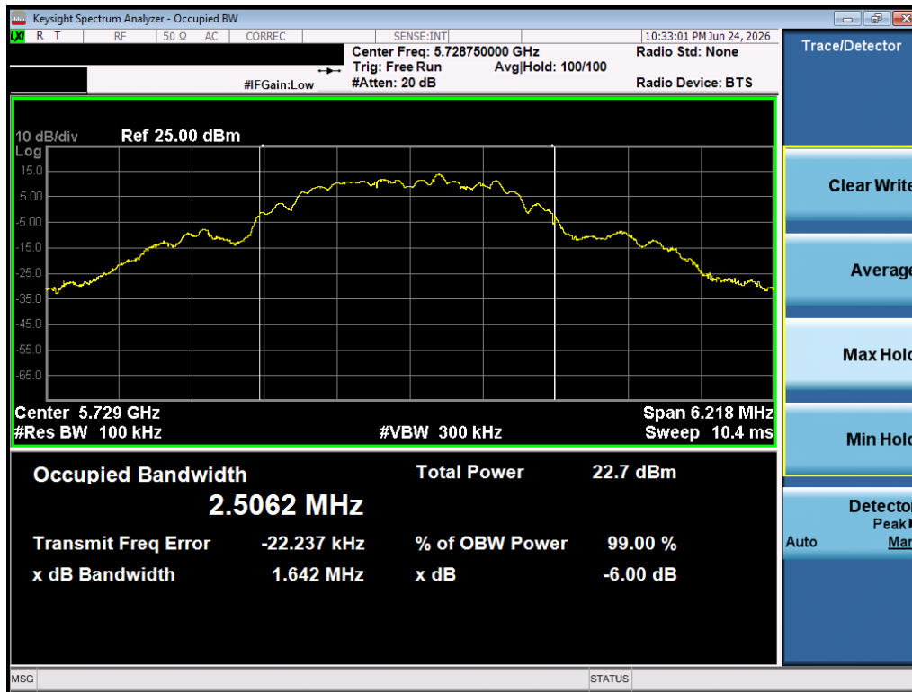
Plot 7-10. 6dB BW (O-QPSK, 5728.75 MHz, 250kbps)
