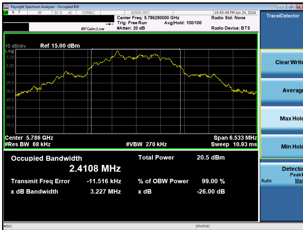
Plot 7-5. 99% OBW (O-QPSK, 5786.25 MHz, 500kbps)
