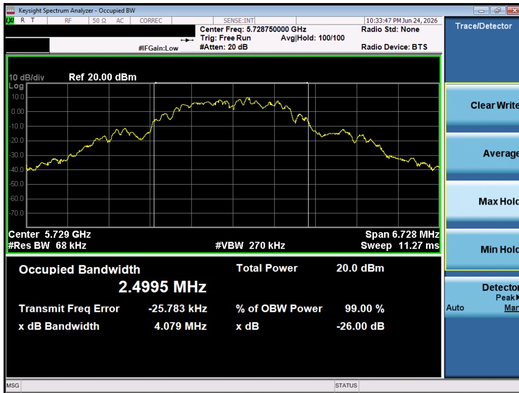
Plot 7-1. 99% OBW (O-QPSK, 5728.75 MHz, 250kbps)
