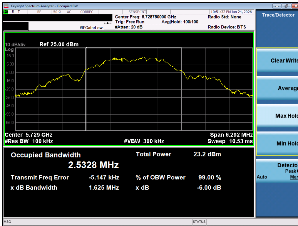
Plot 7-16. 6dB BW (O-QPSK, 5728.75 MHz, 1000kbps)
