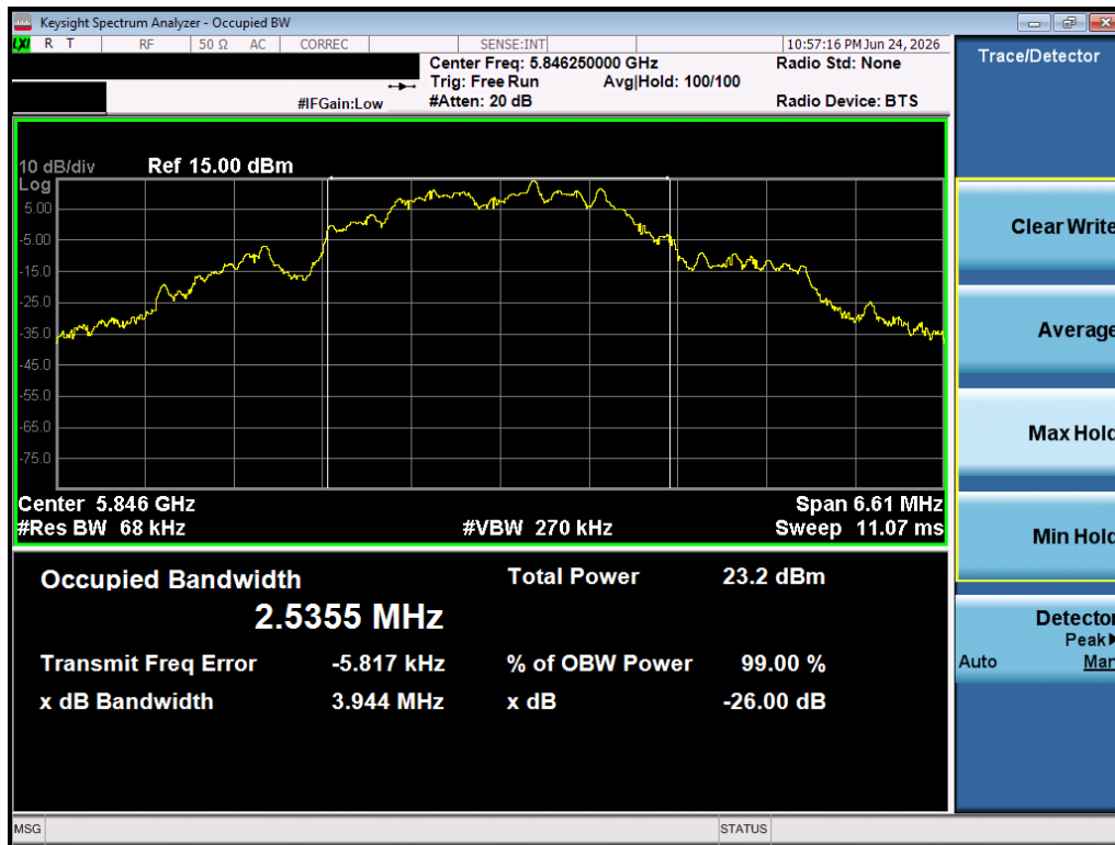
Plot 7-9. 99% OBW (O-QPSK, 5846.25 MHz, 1000kbps)
