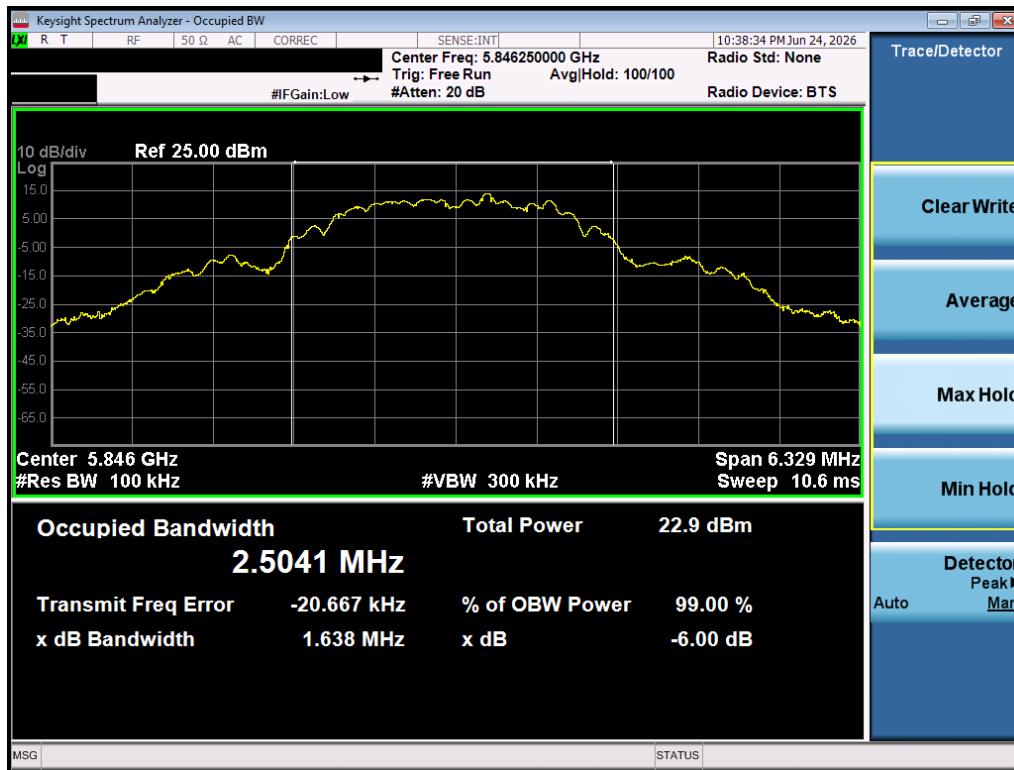
Plot 7-12. 6dB BW (O-QPSK, 5846.25 MHz, 250kbps)
