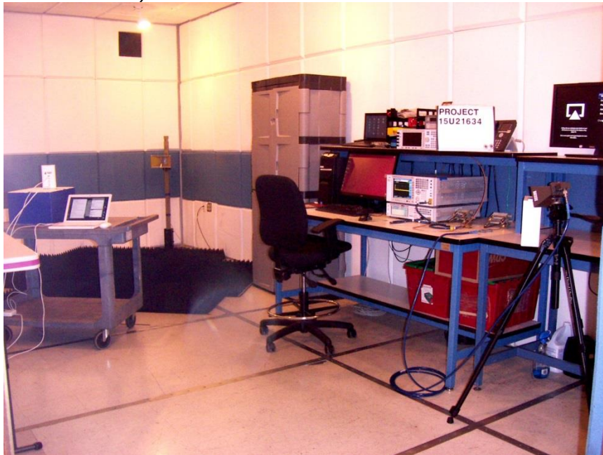
DFS FRONT PHOTO (CLIENT-TO-CLIENT COMMUNICATIONS MODE SETUP)
