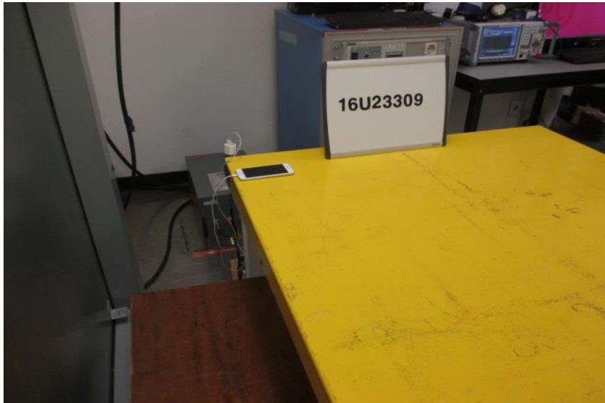
LINE CONDUCTED BACK PHOTO
