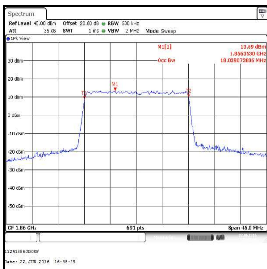
Bottom Channel / 16QAM
