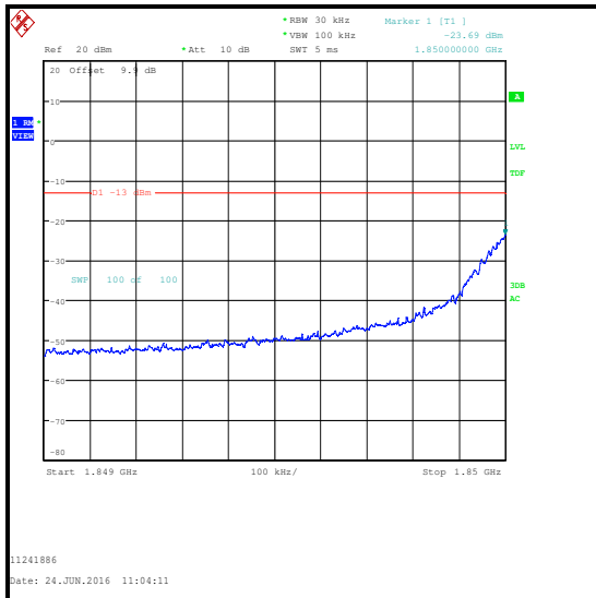
16QAM / 1 RB 0 offset / Lower Band Edge
