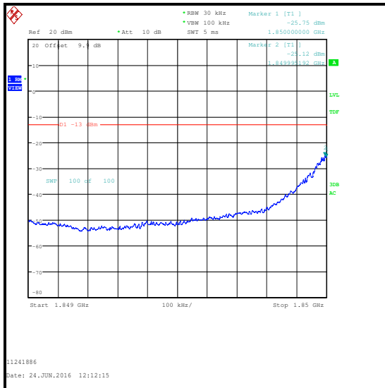
QPSK / 1 RB 0 offset / Lower Band Edge
