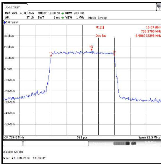
Bottom Channel / 16QAM
