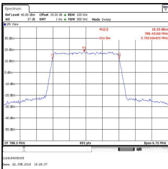
Bottom Channel / 16QAM
