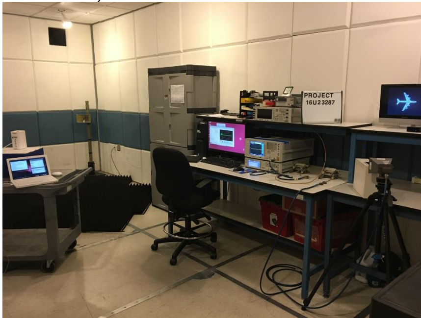
DFS FRONT PHOTO (CLIENT-TO-CLIENT COMMUNICATIONS MODE SETUP)
