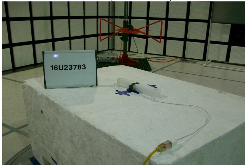
RADIATED FRONT PHOTO (BELOW 1 GHz)
