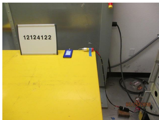
AC LINE CONDUCTED (FRONT)
