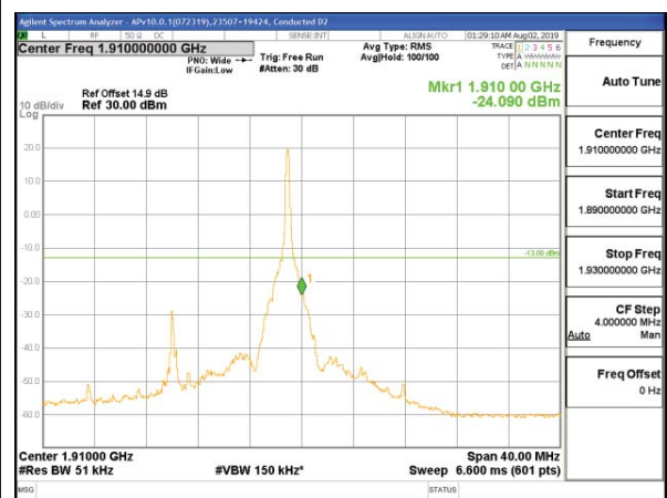
LTE B2 20MHz 16QAM High Channel RB1-99 Marker is wrong
