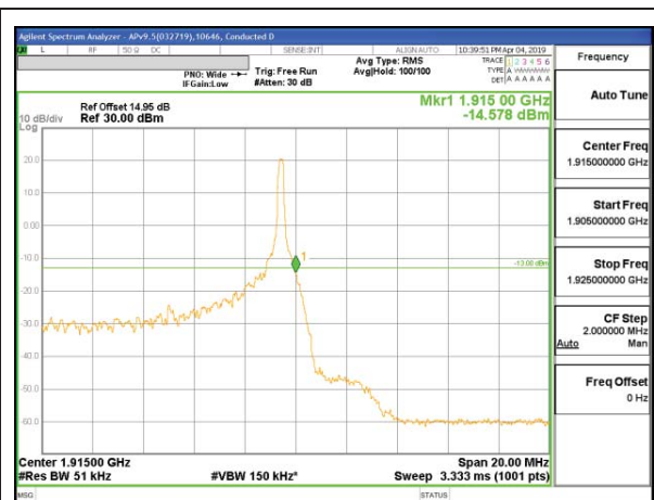
LTE B25 10MHz QPSK High Channel RB1-49
