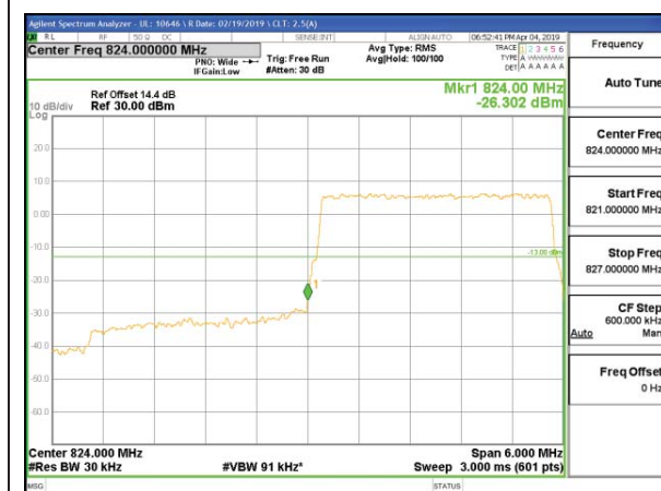
LTE B5 3MHz QPSK Low Channel RB15-0
