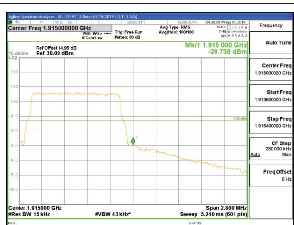
LTE B25 1.4MHz 16QAM High Channel RB6-0
