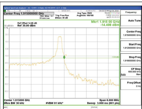
LTE B25 3MHz 16QAM High Channel RB1-14
