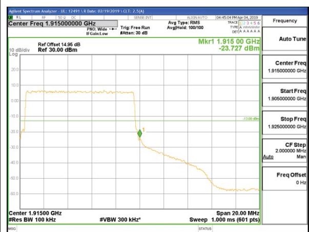
LTE B25 10MHz QPSK High Channel RB50-0
