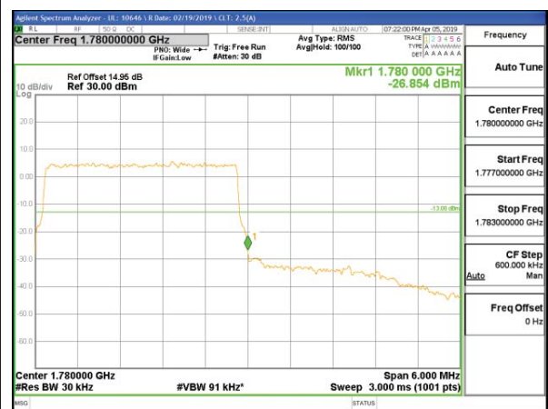
LTE B66 3MHz 16QAM High Channel RB15-0
