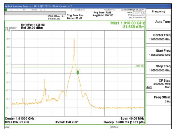
LTE B25 20MHz QPSK High Channel RB1-99
