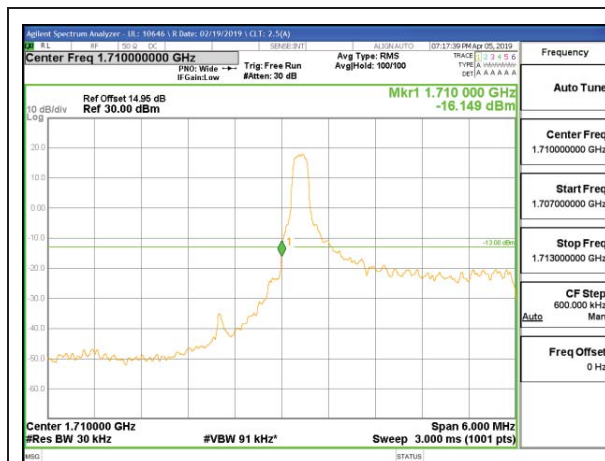
LTE B66 3MHz 16QAM Low Channel RB1-0
