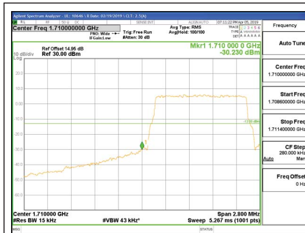
LTE B66 1.4MHz 16QAM Low Channel RB6-0
