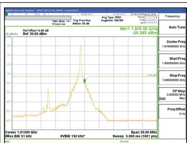
LTE B25 15MHz 16QAM High Channel RB1-74
