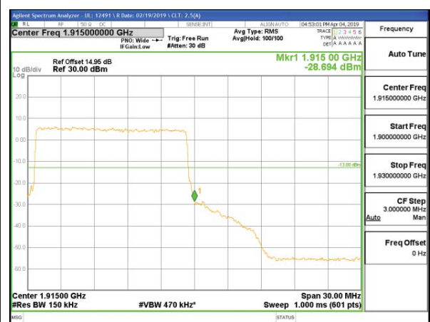
LTE B25 15MHz 16QAM High Channel RB75-0
