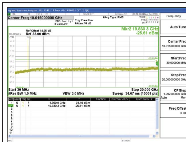
LTE B25 3MHz QPSK Low Channel RB1-0
