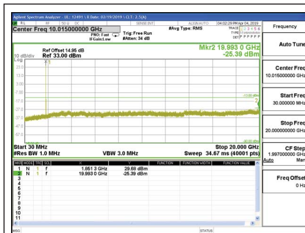
LTE B25 5MHz QPSK Low Channel RB1-0
