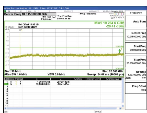
LTE B25 3MHz 16QAM Low Channel RB1-0
