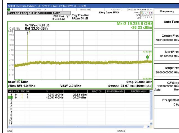
LTE B25 3MHz QPSK High Channel RB1-0
