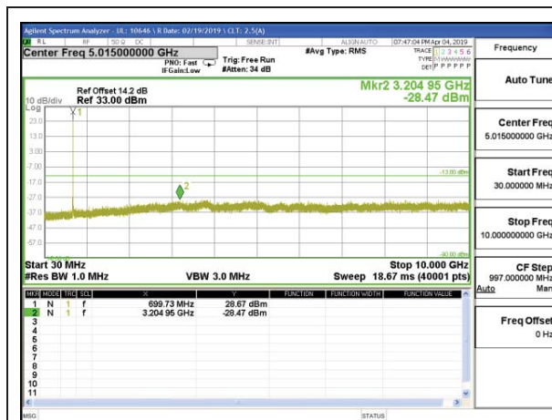
LTE B12 3MHz QPSK Low Channel RB1-0
