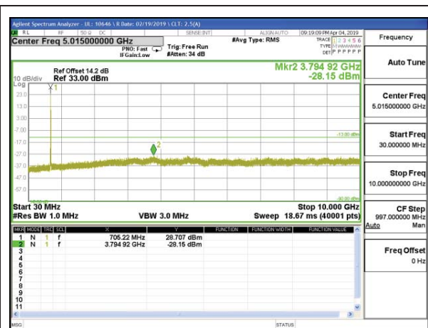
LTE B17 10MHz 16QAM Low Channel RB1-0
