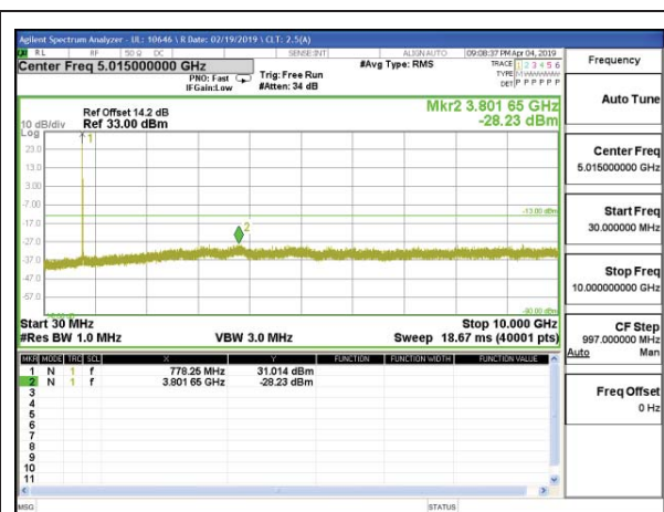
LTE B13 10MHz 16QAM Middle Channel RB1-0
