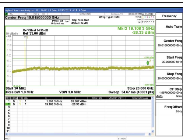
LTE B25 10MHz 16QAM Low Channel RB1-0
