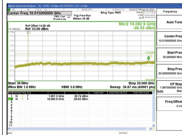
LTE B25 5MHz QPSK Middle Channel RB1-0
