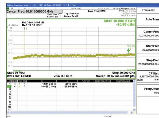
LTE B25 5MHz QPSK High Channel RB1-0
