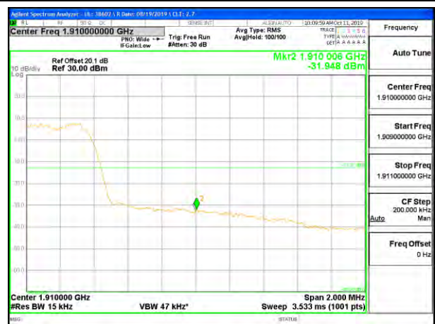
CDMA BC1 1xEV-DO Rev A High Channel
