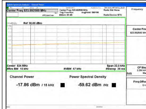
CDMA BC0 1xEV-DO Rev A Low Channel
