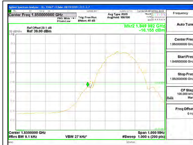
GSM 1900 GPRS Low Channel
