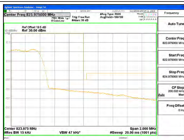
CDMA BC10 1xEV-DO Rev A High Channel, RBW=1% of EBW
