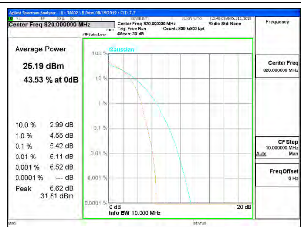
CDMA BC10 1xEV-DO Rev A Middle Channel
