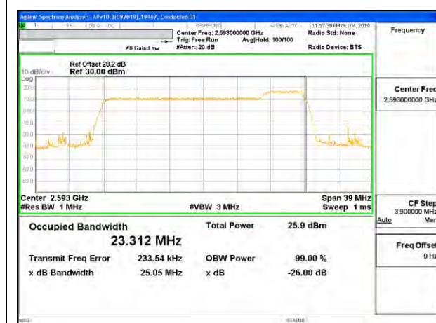
LTE B41 20MHz + 5MHz 16QAM RB100-0 + RB25-0
