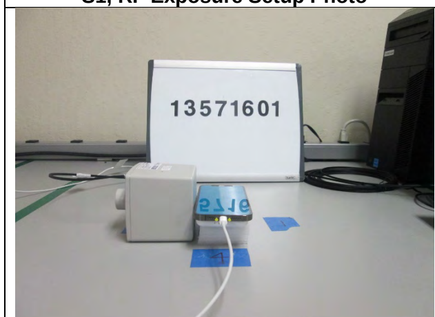
S3, RF Exposure Setup Photo
