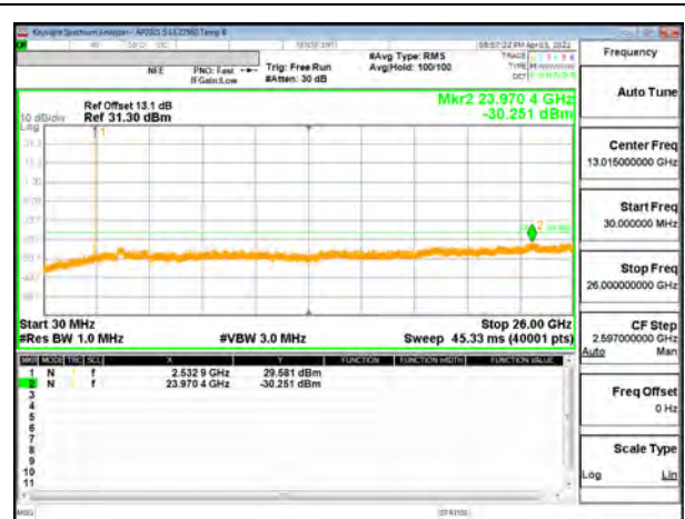
5G NR n7 5MHz BPSK Middle Channel RB1-1
