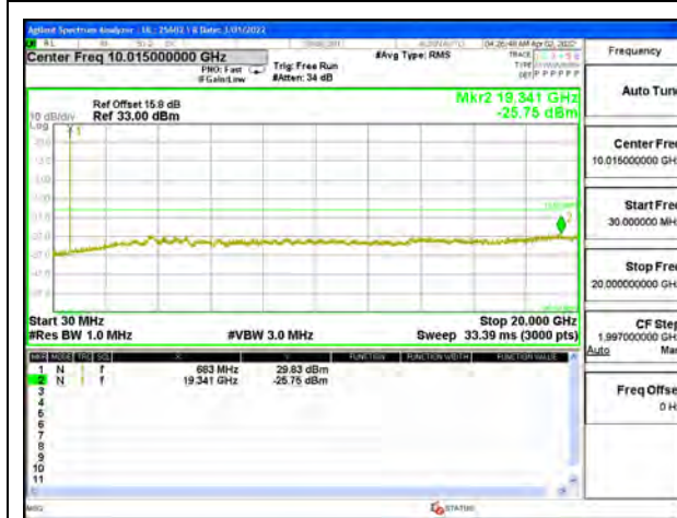
LTE B71 15MHz QPSK High Channel RB1-0
