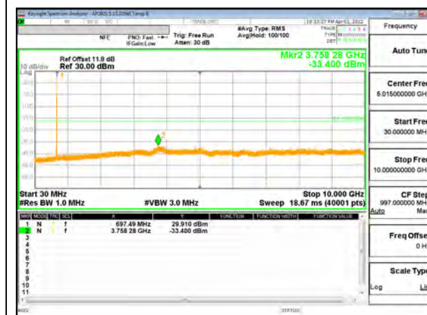
5G NR n71 15MHz BPSK High Channel RB1-78
