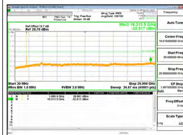
5G NR n70 15MHz BPSK Middle Channel RB1-0
