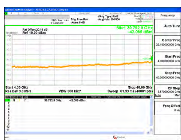
LTE B48 10MHz QPSK High Channel RB1-0 (4G to 40G)
