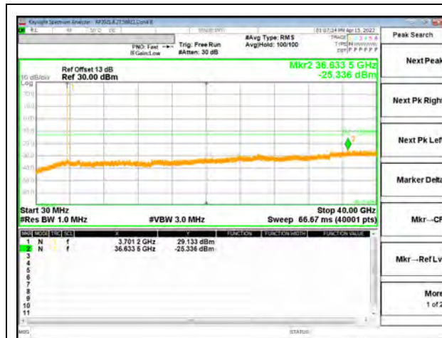
5G NR n77 10MHz BPSK Low Channel RB1-0
