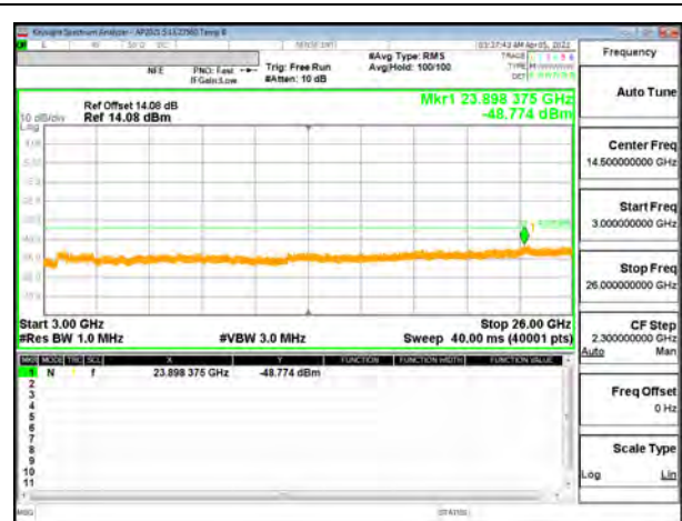
5G NR n30 5MHz BPSK Low Channel RB1-1 (3G to 26G)
