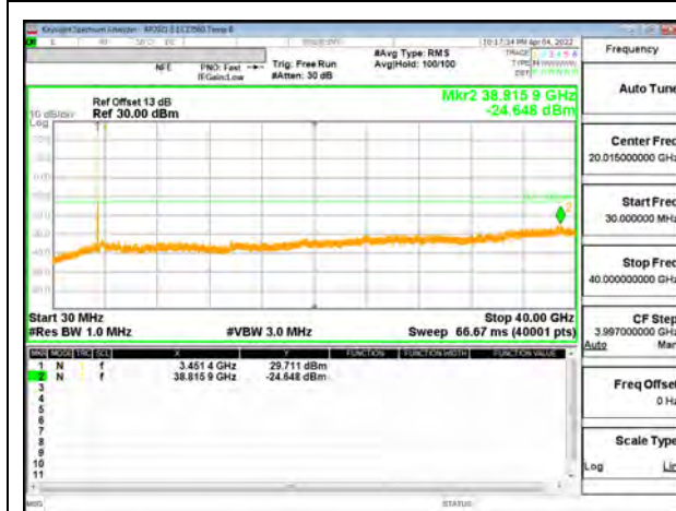
5G NR n77 40MHz BPSK Low Channel RB1-0
