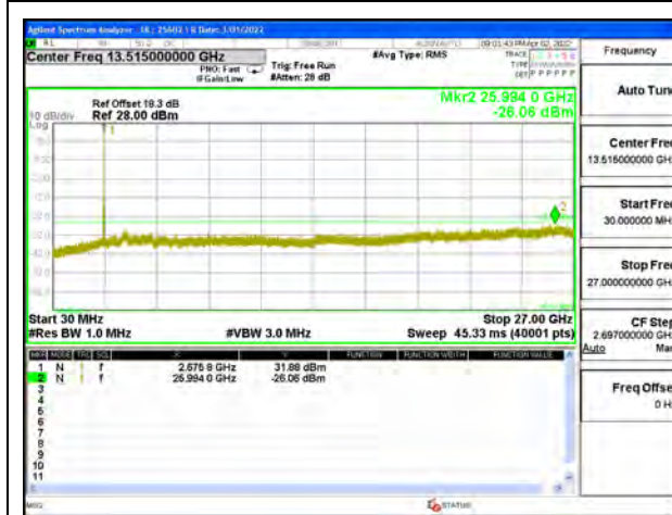
LTE B41 15MHz QPSK High Channel RB1-0
