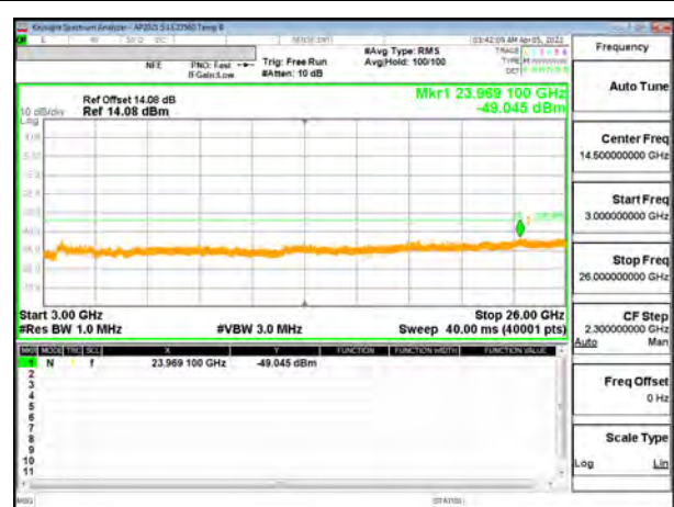
5G NR n30 10MHz BPSK High Channel RB1-0 (3G to 26G)
