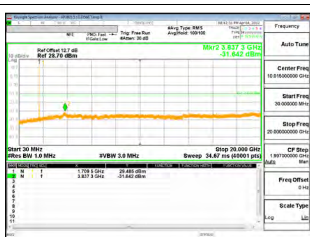
5G NR n70 10MHz BPSK High Channel RB1-51
