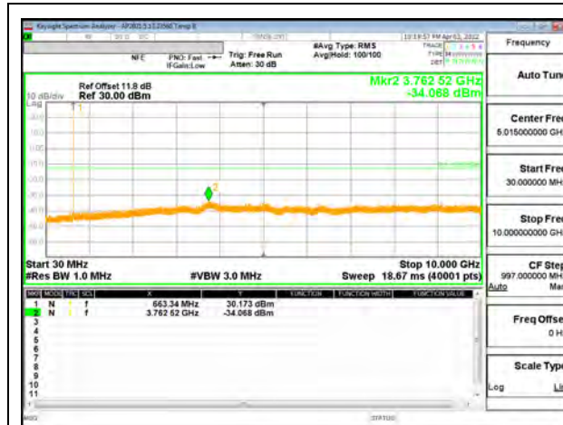
5G NR n71 5MHz BPSK Low Channel RB1-0
