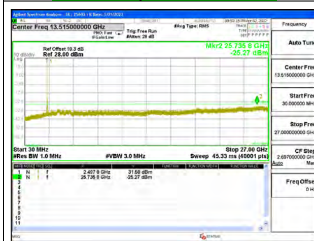
LTE B41 15MHz QPSK Low Channel RB1-0
