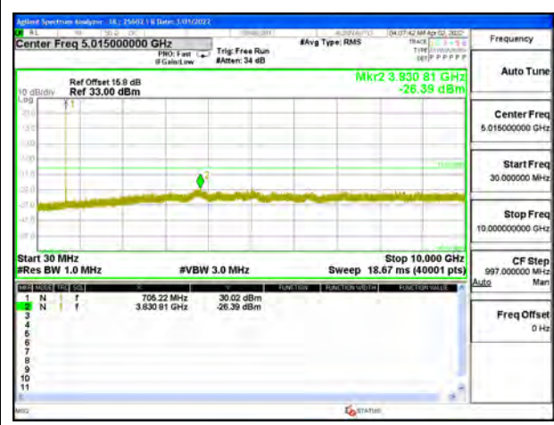
LTE B17 10MHz QPSK Low Channel RB1-0
