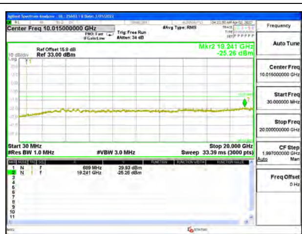
LTE 71 10MHz QPSK High Channel RB1-0
