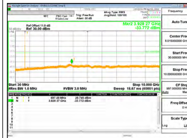
5G NR n71 5MHz BPSK High Channel RB1-24
