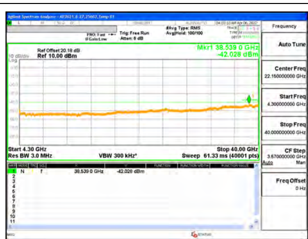
LTE B48 5MHz QPSK High Channel RB1-0 (4G to 40G)
