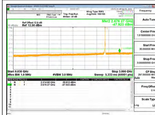
5G NR n30 5MHz BPSK High Channel RB1-24 (30M to 3G)
