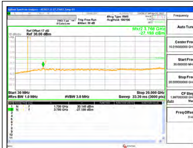
LTE B66 1.4MHz QPSK Low Channel RB1-0
