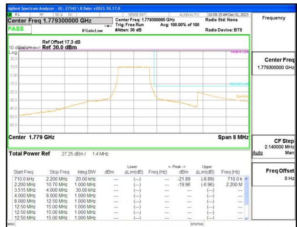
LTE B66 1.4MHz QPSK High Channel RB6-0
