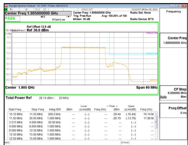
5G NR n25 20MHz BPSK High Channel RB100-0
