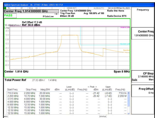
LTE B25 1.4MHz QPSK High Channel RB6-0
