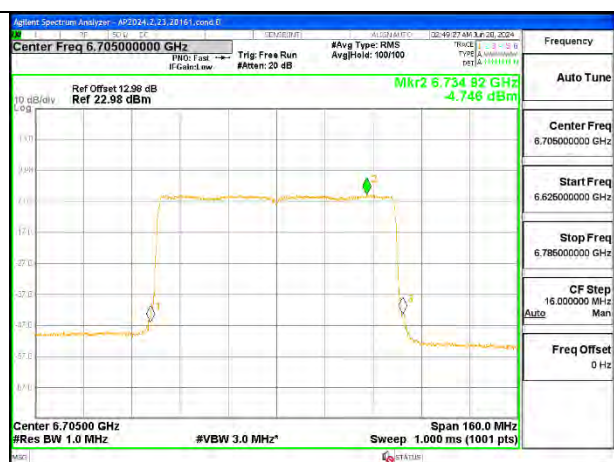
80MHz - Mid Channel – SU (UNII-7) – Ant 5
