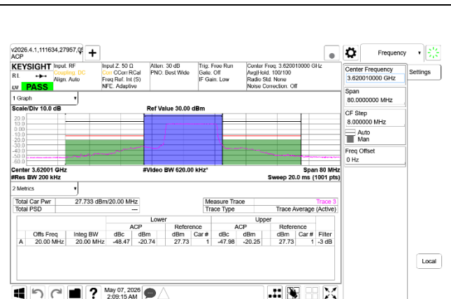
5G NR n48 15MHz BPSK Middle Channel RB36-0 (3622.5MHz), Ant7+Ant8
