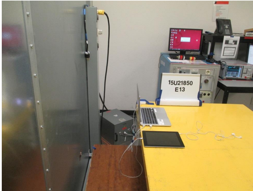
EUT WITH LAPTOP LINE CONDUCTED BACK PHOTO
