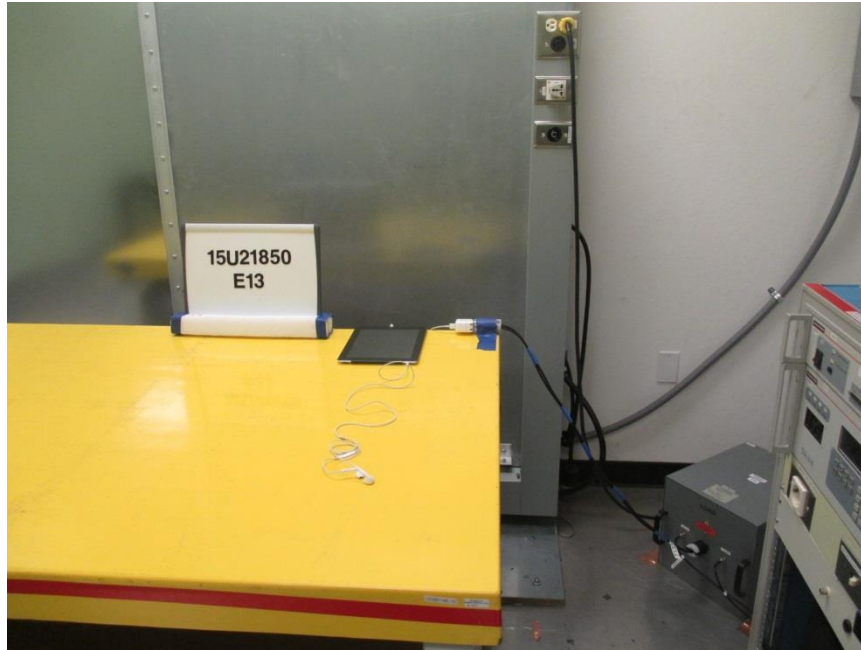
EUT ONLY LINE CONDUCTED FRONT PHOTO
