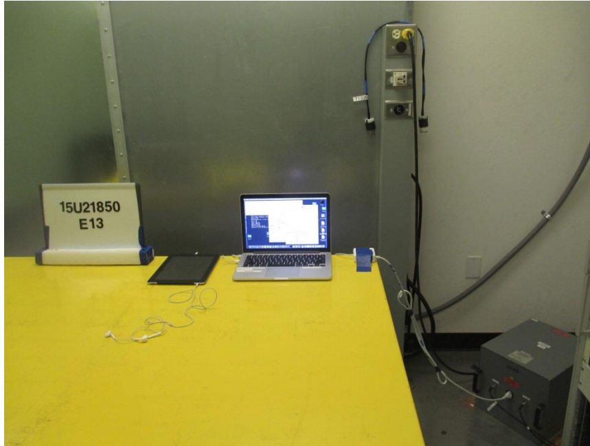
EUT WITH LAPTOP LINE CONDUCTED FRONT PHOTO
