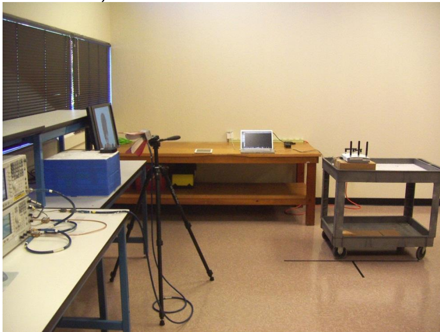
DFS FRONT PHOTO (CLIENT-TO-CLIENT COMMUNICATIONS MODE SETUP)
