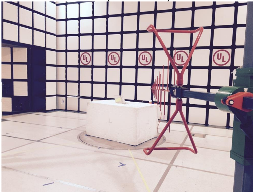
RADIATED BACK PHOTO (BELOW 1 GHz)
