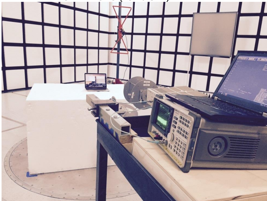
RADIATED FRONT PHOTO (18-26 GHz)
