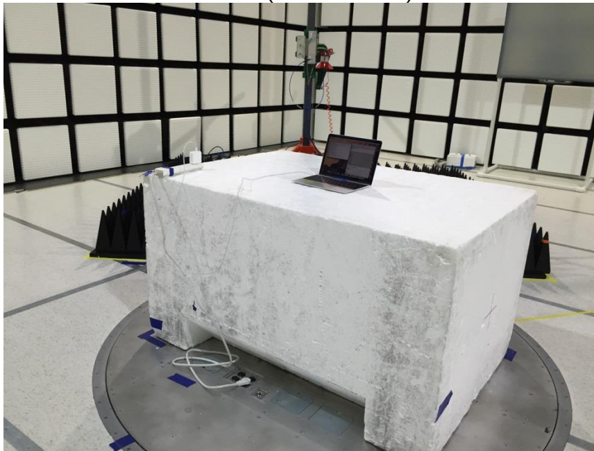
RADIATED FRONT PHOTO (ABOVE 1 GHz)
