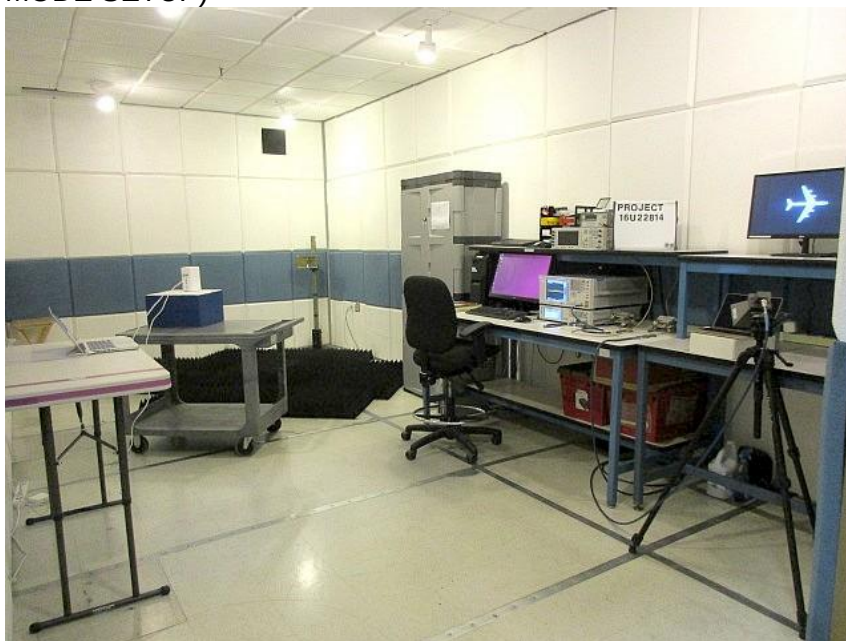
DFS FRONT PHOTO (CLIENT-TO-CLIENT COMMUNICATIONS MODE SETUP)
