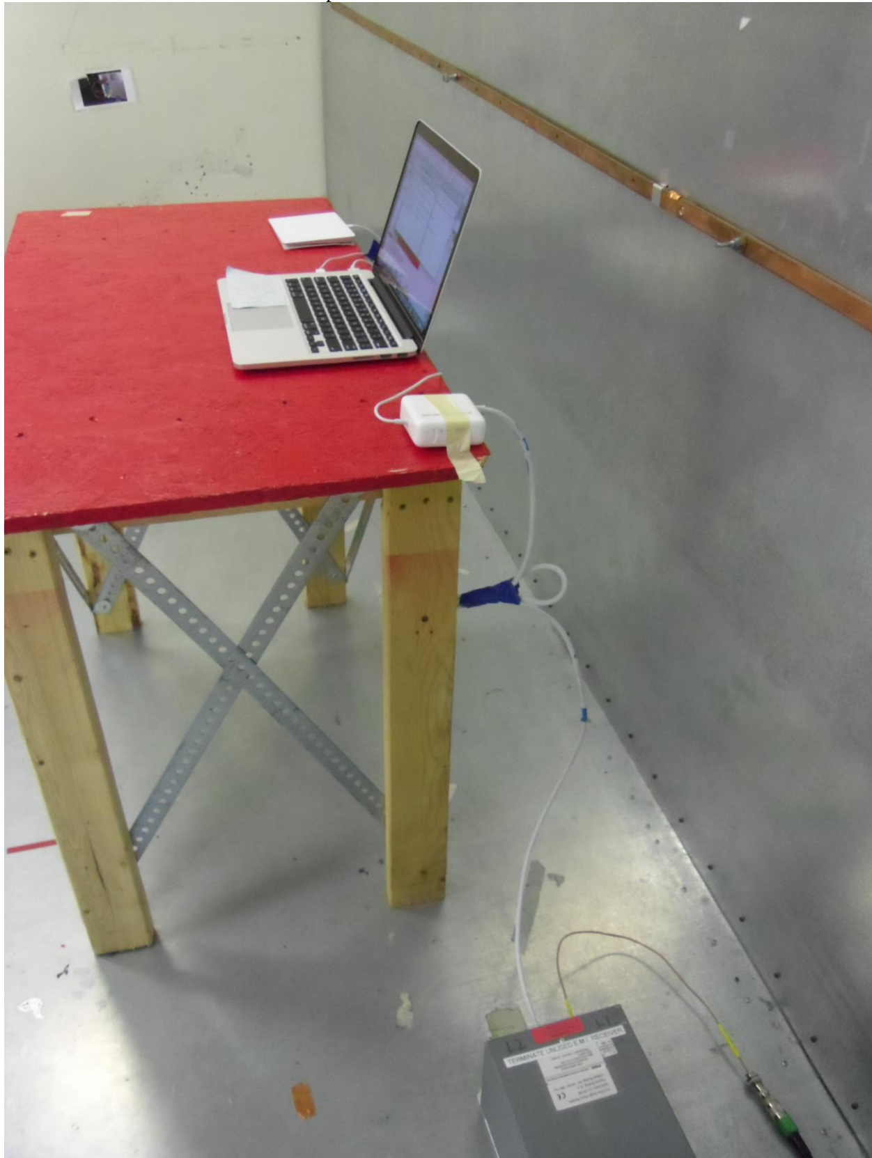
AC Line Conducted Emissions Setup 1
