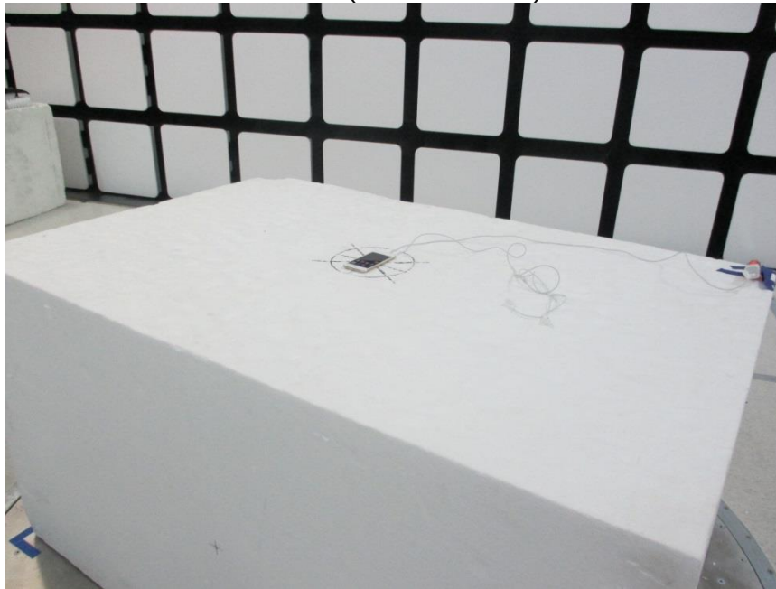
RADIATED FRONT PHOTO (BELOW 1 GHz)
