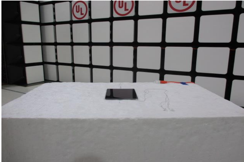
RADIATED FRONT PHOTO (BELOW 1 GHz)
