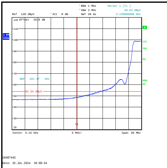
Lower Band Edge Average Measurement
