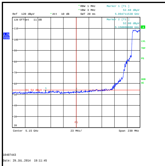
Lower Band Edge Peak Measurement
