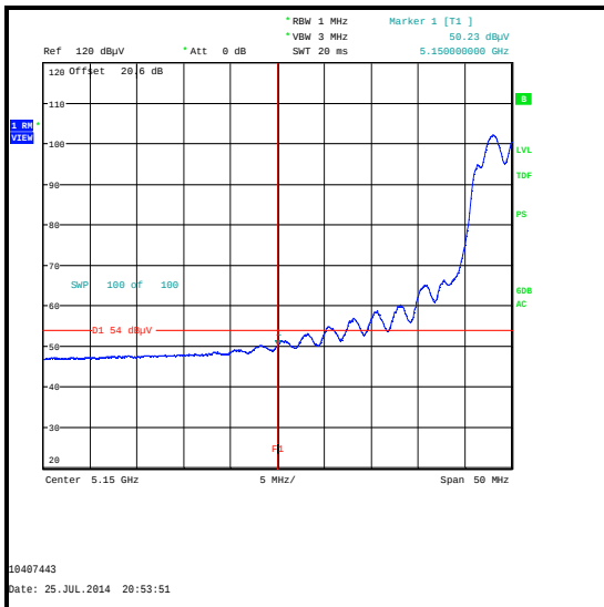
Lower Band Edge Average Measurement
