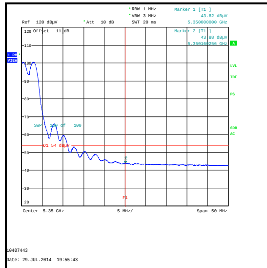
Upper Band Edge Average Measurement
