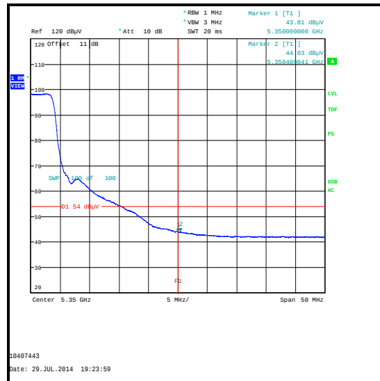
Upper Band Edge Average Measurement
