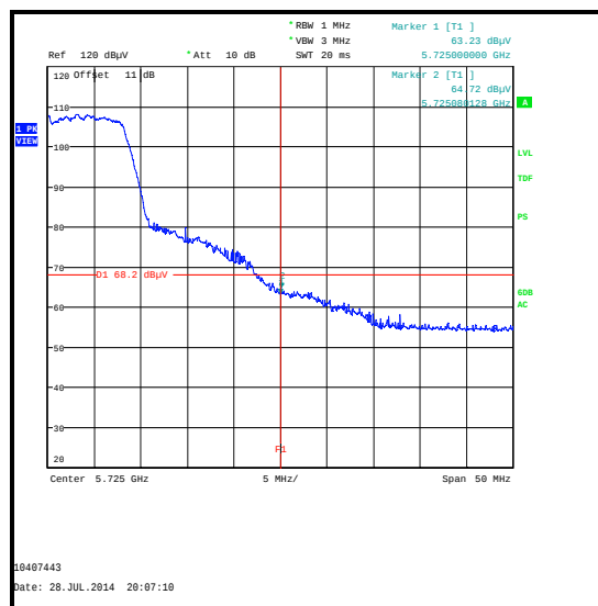
Upper Band Edge Measurement
