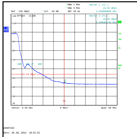
Upper Band Edge Average Measurement
