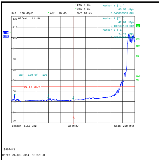
Lower Band Edge Average Measurement
