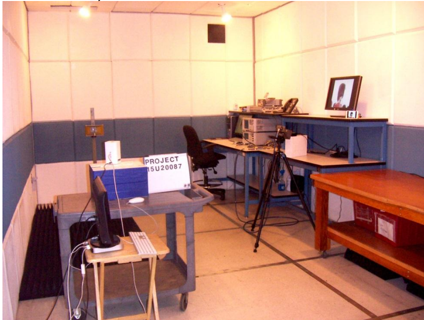
DFS FRONT PHOTO (CLIENT-TO-CLIENT COMMUNICATIONS MODE SETUP)
