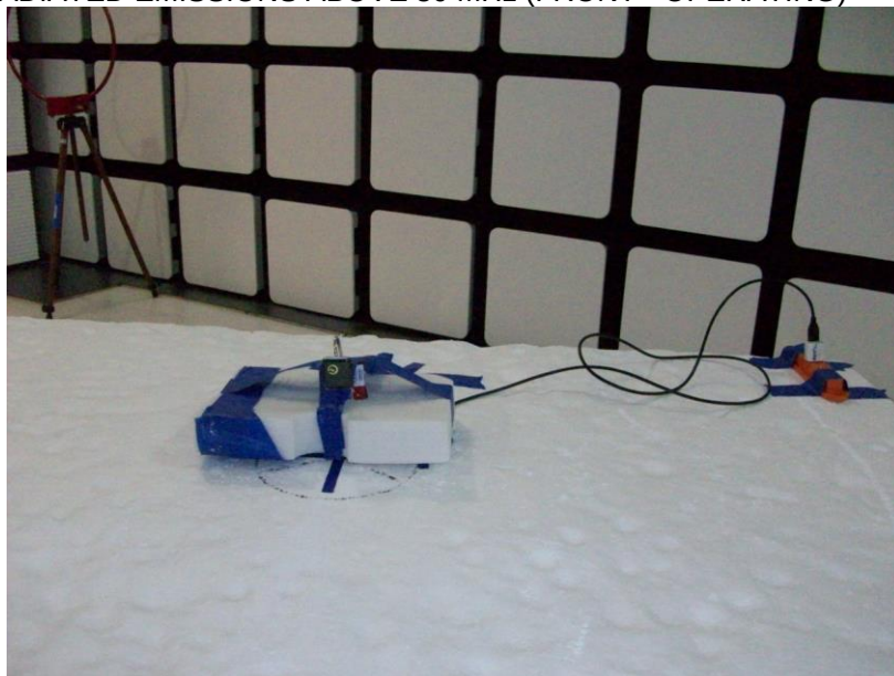
RADIATED EMISSIONS ABOVE 30 MHz (FRONT - OPERATING)
