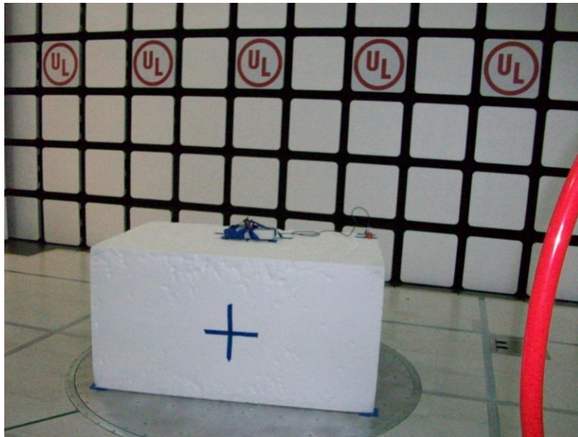
RADIATED EMISSIONS BELOW 30MHz (FRONT - OPERATING)
