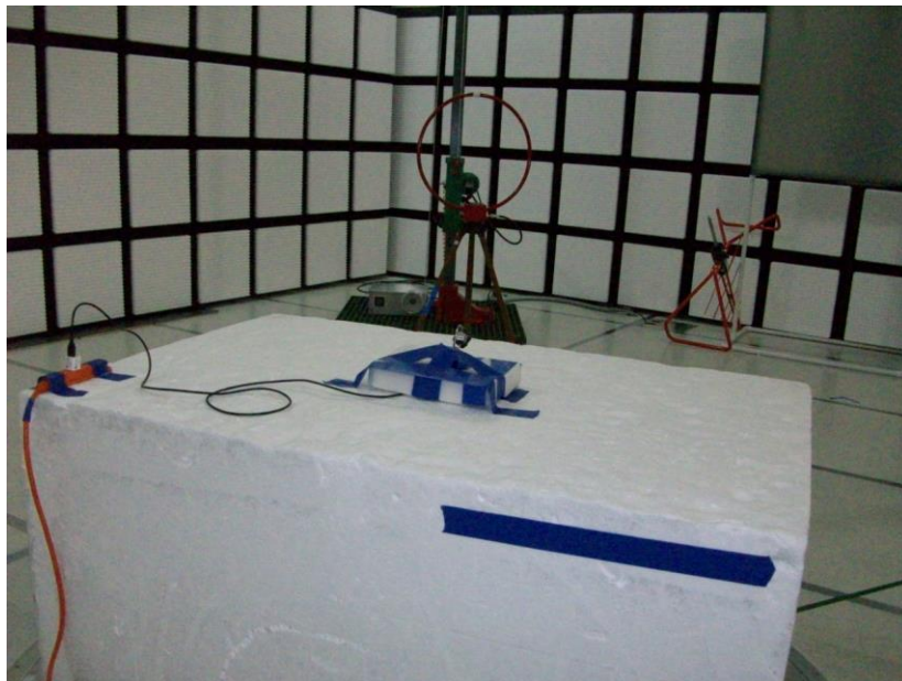
RADIATED EMISSIONS BELOW 30MHz (BACK - OPERATING)
