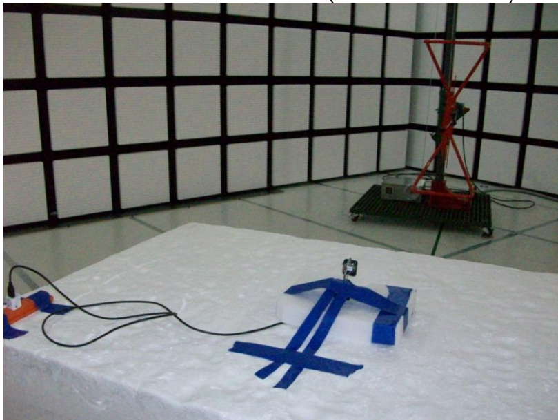
RADIATED EMISSIONS ABOVE 30 MHz (BACK - OPERATING)
