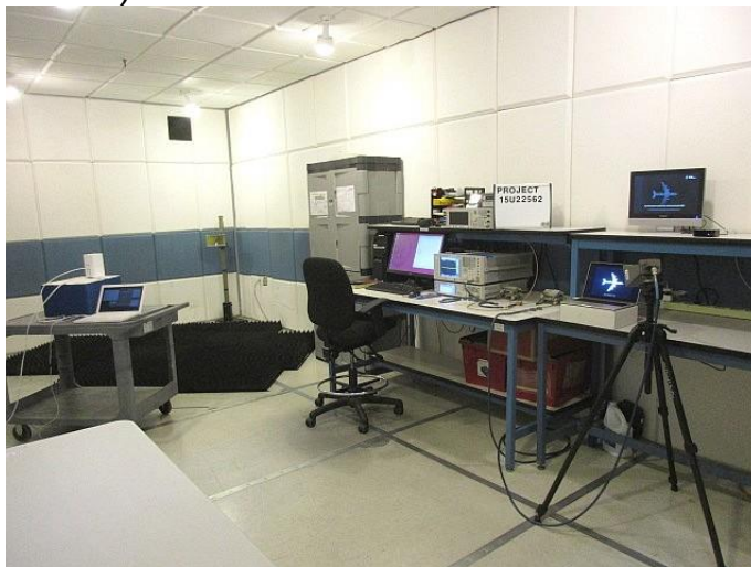
DFS FRONT PHOTO (CLIENT-TO-CLIENT COMMUNICATIONS MODE SETUP)
