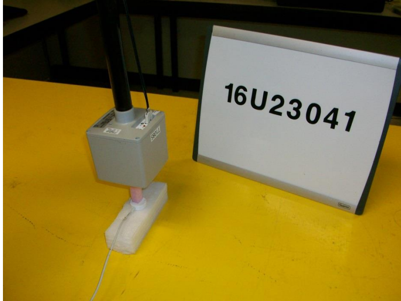
TOP, RF EXPOSURE SETUP PHOTO
