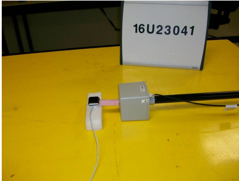
S3, RF EXPOSURE SETUP PHOTO
