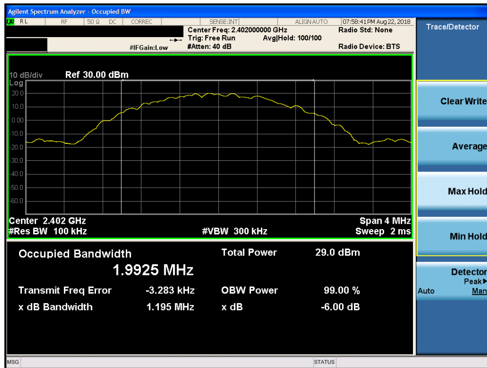
Plot 7-4. 6dB Bandwidth Plot (Bluetooth (LE), 2Mbps, ePA – Ch. 0, Antenna 0)
