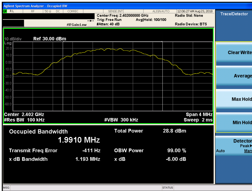
Plot 7-10. 6dB Bandwidth Plot (Bluetooth (LE), 2Mbps, ePA – Ch. 0, Antenna 1)
