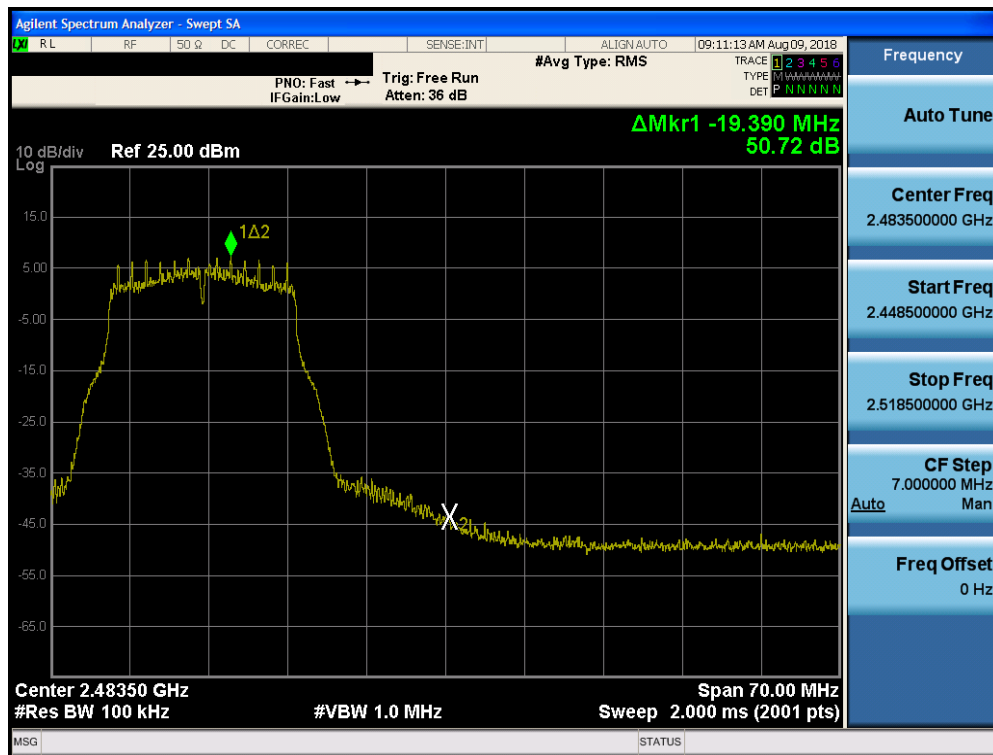
Plot 7-84. Band Edge Plot SISO Core 0 (802.11g - Ch. 11)
