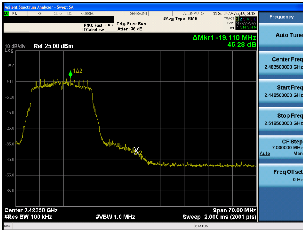
Plot 7-100. Band Edge Plot SISO Core 1 Primary (802.11n (2.4GHz) – Ch. 11)
