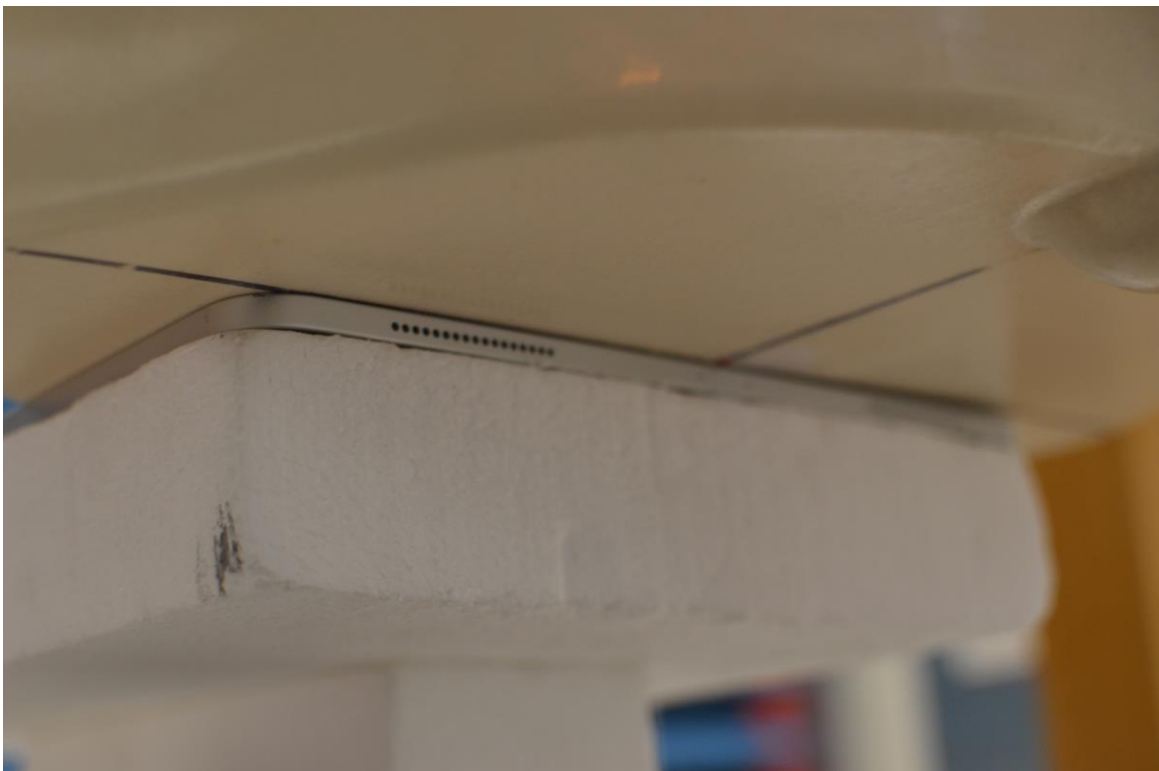
SAR Test Setup Photo 2: Back Side at 0 mm (for Antenna WF8, WF7, and Upper testing)
