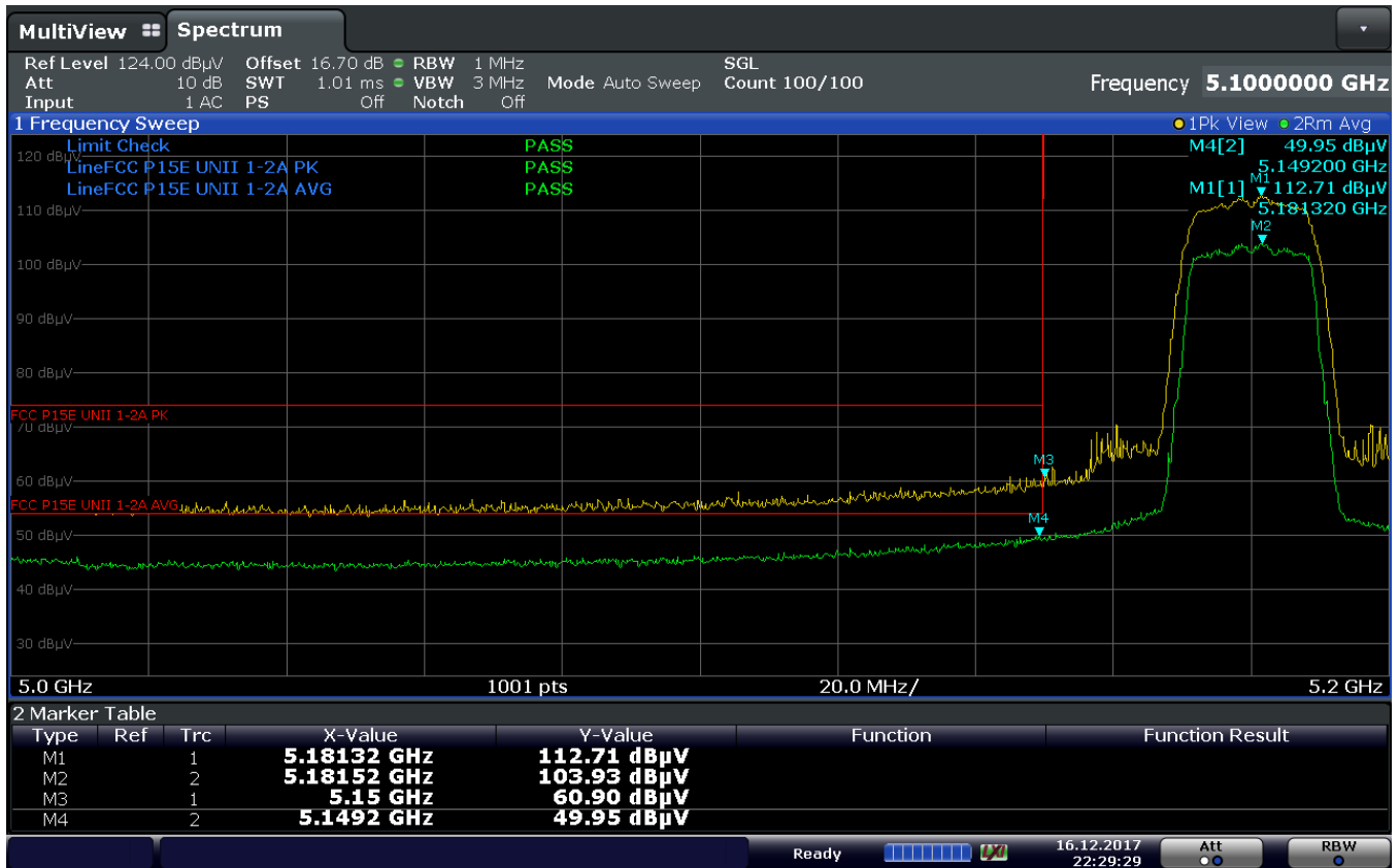
Plot 7-325. Radiated Restricted Lower Band Edge Measurement SISO ANT2 (Average & Peak UNII Band 1)
