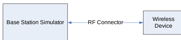
Figure 8-2 Power Measurement Setup
