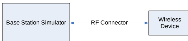
Figure 8-1 Power Measurement Setup
