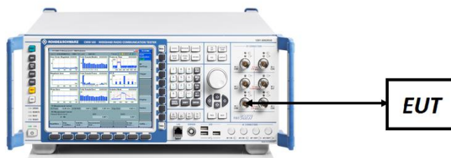
Figure 7-5. ERP/EIRP Measurement Setup
