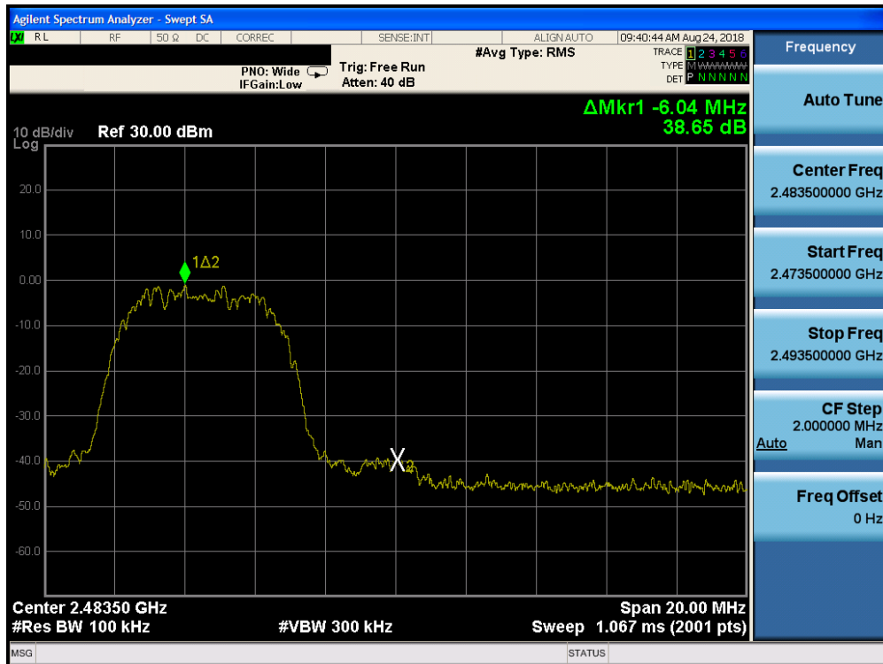
Plot 7-66. Band Edge Plot ANT2 (Bluetooth (HDR8, ePA), 8Mbps – Ch. 75)
