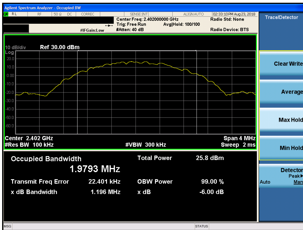
Plot 7-4. 6dB Bandwidth Plot ANT0 (Bluetooth (LE), 2Mbps, ePA – Ch. 0)
