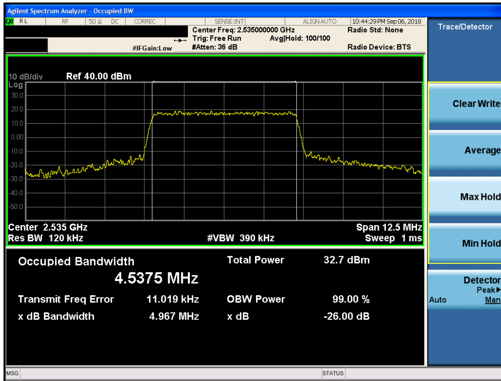
Plot 7-73. Occupied Bandwidth Plot (Band 7 – 5.0MHz QPSK – RB Size 25)
