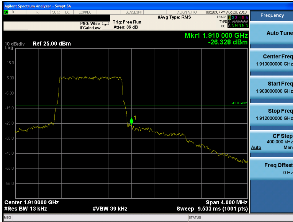
Plot 7-246. Upper Band Edge Plot (Band 2 – 1.4MHz QPSK – RB Size 6)
