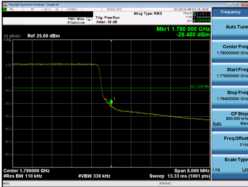
Plot 7-234. Upper Band Edge Plot (Band 66 – 10.0MHz QPSK – RB Size 50)
