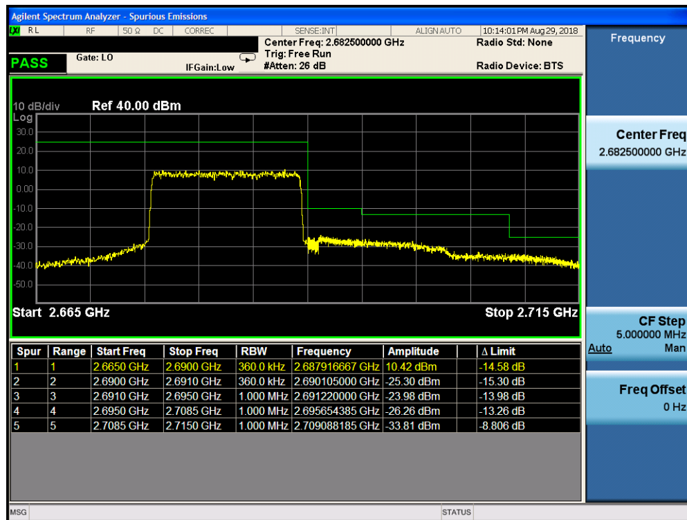
Plot 7-313. Upper ACP Plot (Band 41 – 15.0MHz QPSK – RB Size 75)
