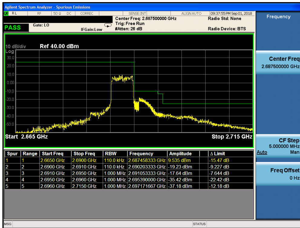
Plot 7-309. Upper ACP Plot (Band 41 – 5.0MHz QPSK – RB Size 25)
