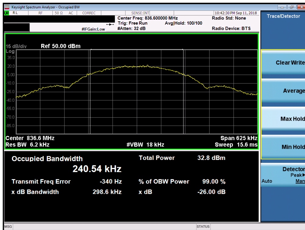
Plot 7-2. Occupied Bandwidth Plot (EDGE850 Mode)
