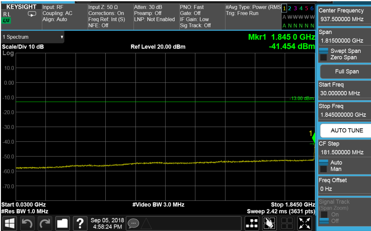
Plot 7-44. Conducted Spurious Plot (PCS WCDMA Mode - Low Channel)
