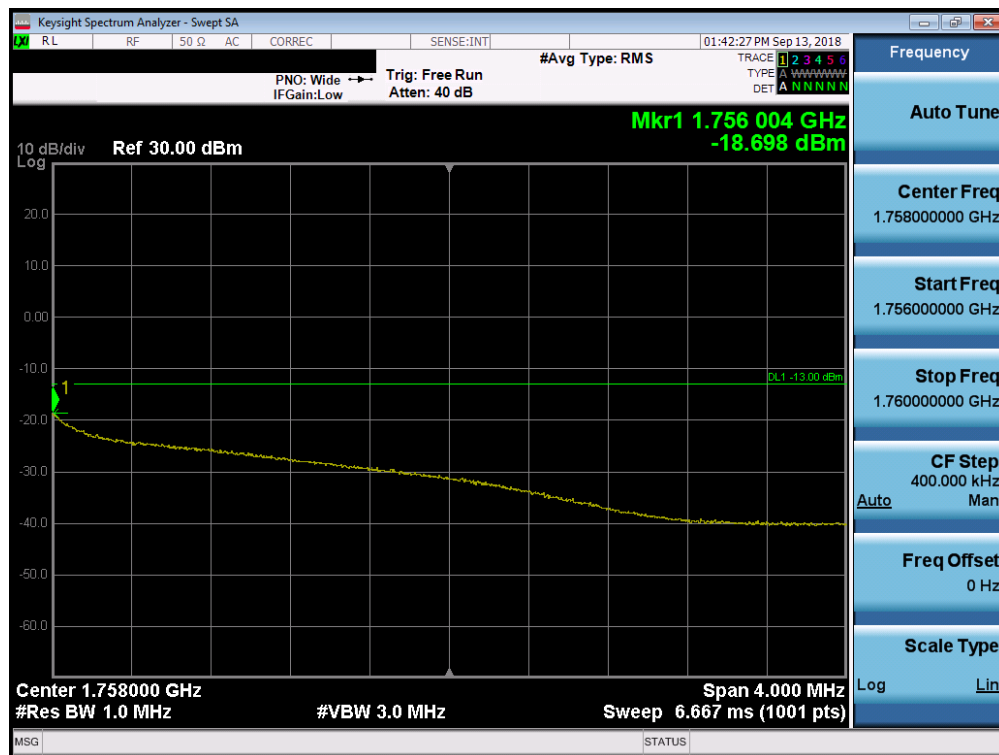
Plot 7-64. 4MHz Span Plot (AWS WCDMA Mode - High Channel)
